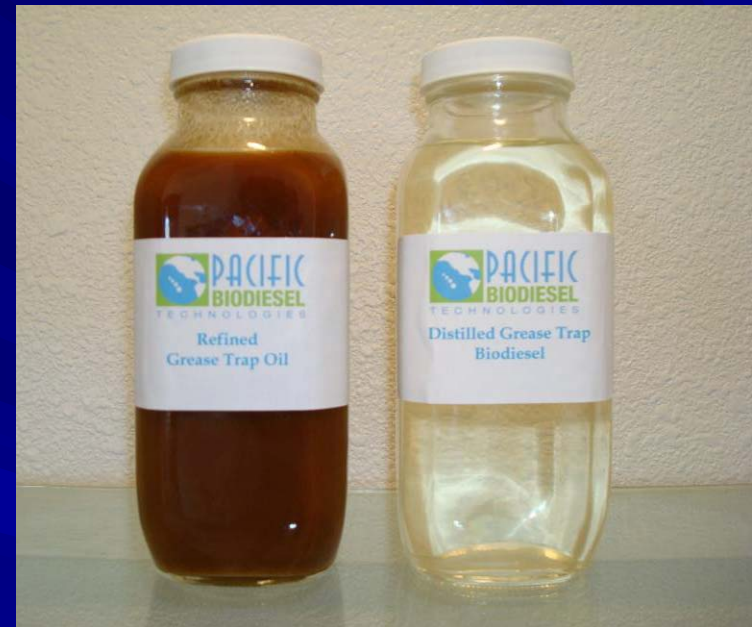
Separated Grease Trap Oil and Finished Grease Trap Biodiesel
