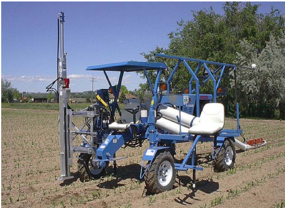
Figure 12. The Coachella Valley Resource Conservation District “Salt Sniffer,” used to measure soil salinity (photo: Scott Lesch, U.S. Department of Agriculture)
