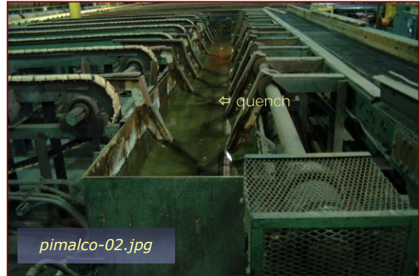
Photo #2: Aerospace Bldg – Extrusion Press Quench Taken By: Greg V. Arthur Date: 08/11/09
