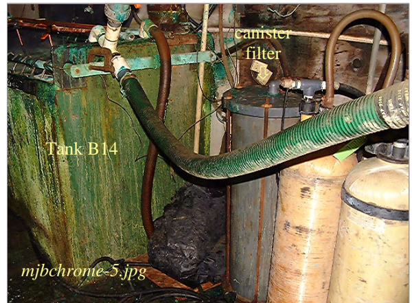
Photo: Nickel Tank B14 and outside filter Taken By: Greg V. Arthur Date: 04/17/07
