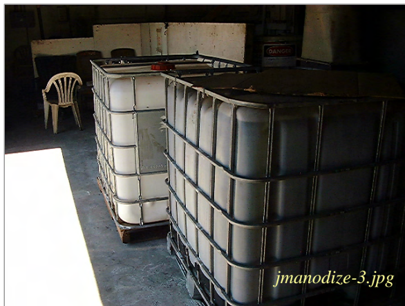
Photo: Totes with spent anodizing solutions Taken By: Greg V. Arthur Date: 09/06/06
