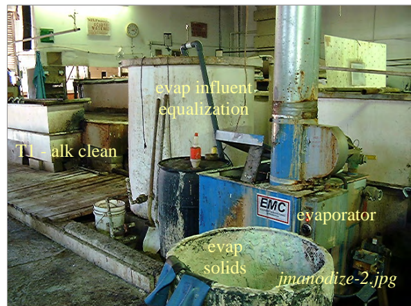
Photo: Evaporator and EQ for spent alkalines Taken By: Greg V. Arthur Date: 09/06/06
