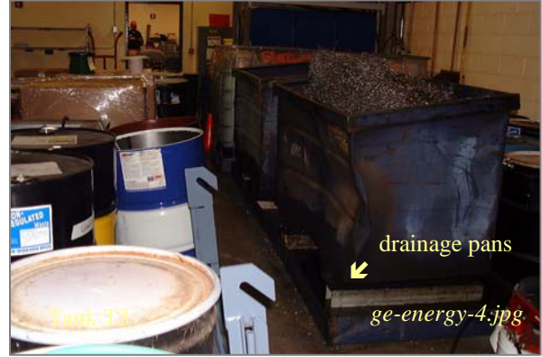
Photo: Chip Reclaim Drainage Pans Taken By: Greg V. Arthur Date: 11/27/07
