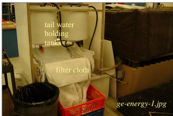
Photo: Vibratory Deburring Tail Water Filtering Taken By: Greg V. Arthur Date: 11/27/07
