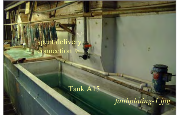
Photo: Spent delivery connection to batch treat Taken By: Greg V. Arthur Date: 10/09/07
