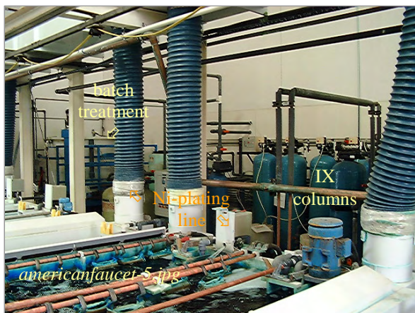
Photo: Ion Exchange Behind Nickel Plating Line Taken By: Greg V. Arthur Date: 05/03/07
