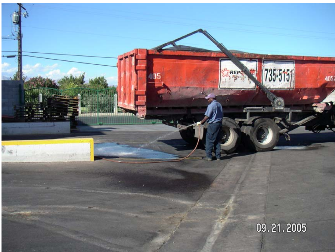
Photo 2. Roll-off container is leaking.
