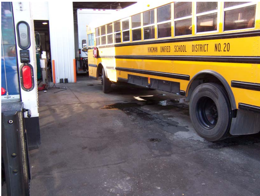
Photo 3. Apparent leakage under bus being maintained outside of shop area.
