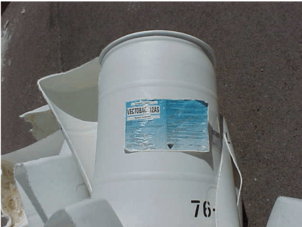
Photo 18. Vector Control facility: Empty drums of larvicide had been cut open in an uncontained location and residue spilled to the pavement.
