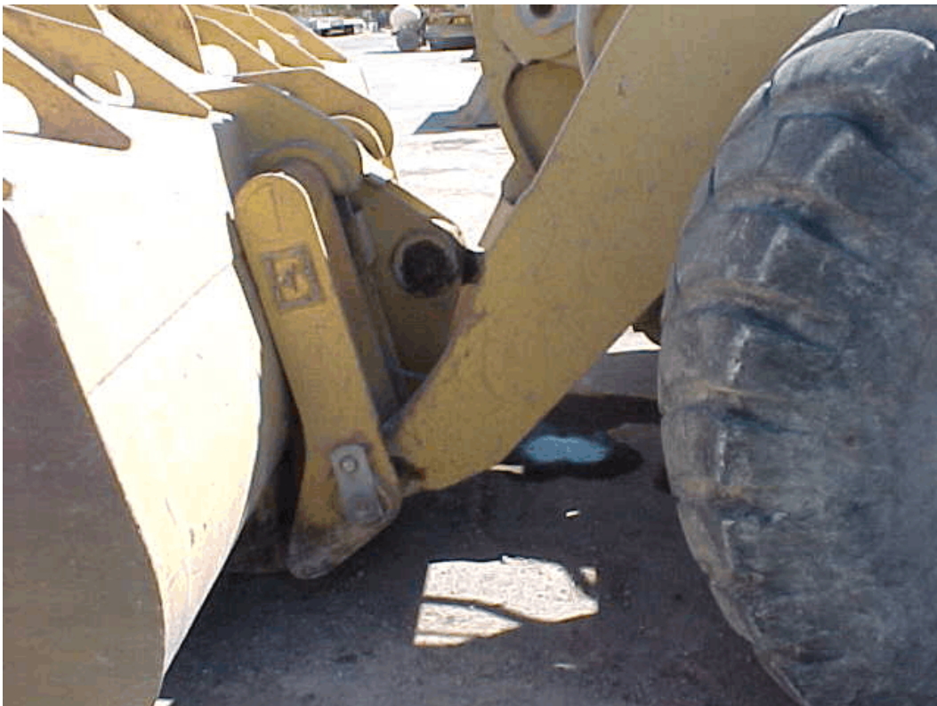
Photo 14. Fleet (secondary) facility: Front loader with an active leak.
