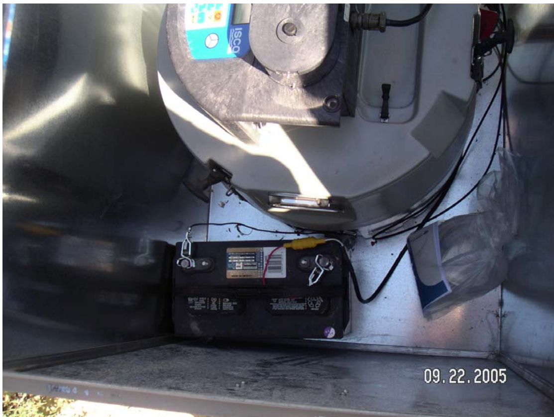
Photo 12. Meadows Detention Basin - marine battery in sampler.
