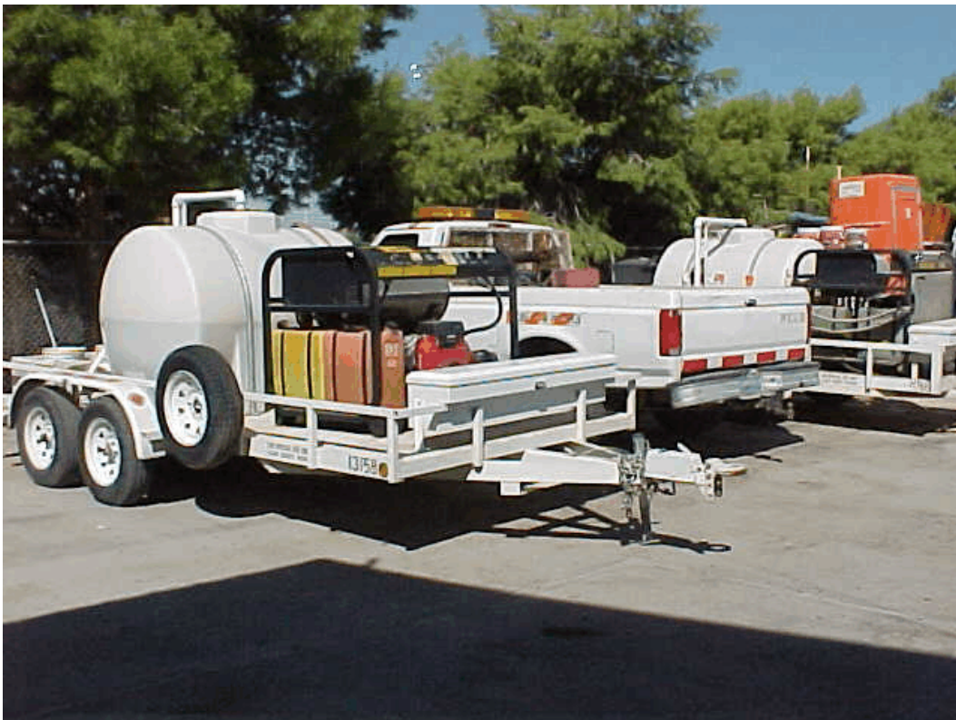
Photo 4. Fleet (primary) facility: Power washer for trucks.
