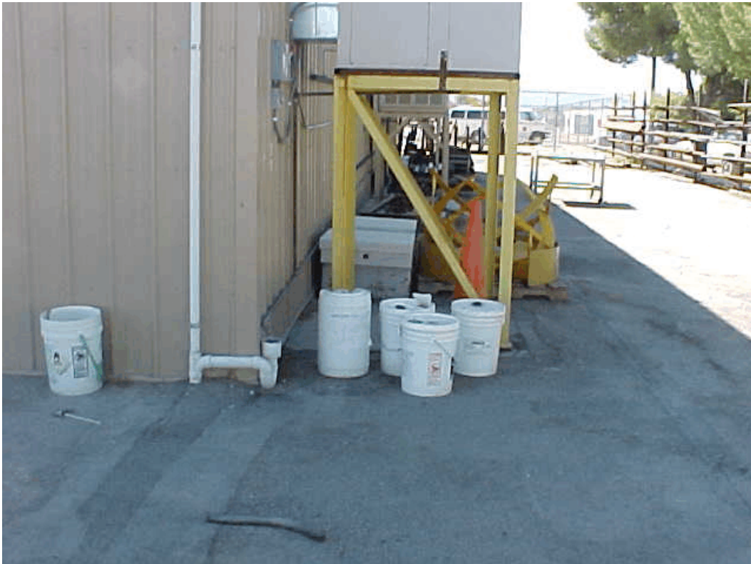
Photo 3. Fleet (primary) facility: Four uncovered and uncontained 5-gallon pails of truck wash chemical.
