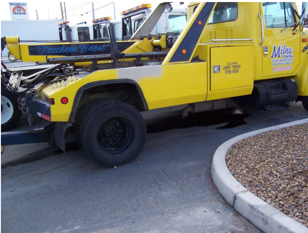
Photo 2. Oil leaking under tow truck stored in the parking area.
