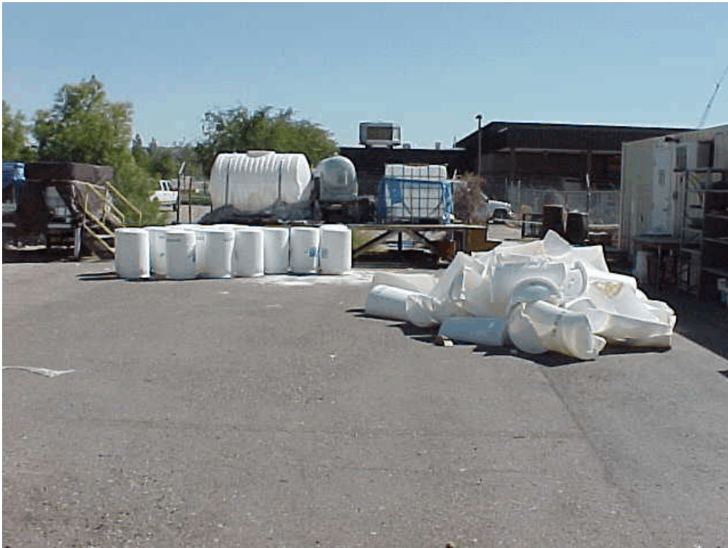
Photo 17. Vector Control facility: Empty drums of larvicide had been cut open in an uncontained location and residue spilled to the pavement.
