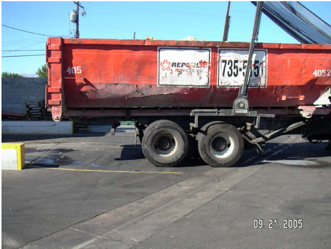
Photo 1. Roll-off container is leaking.
