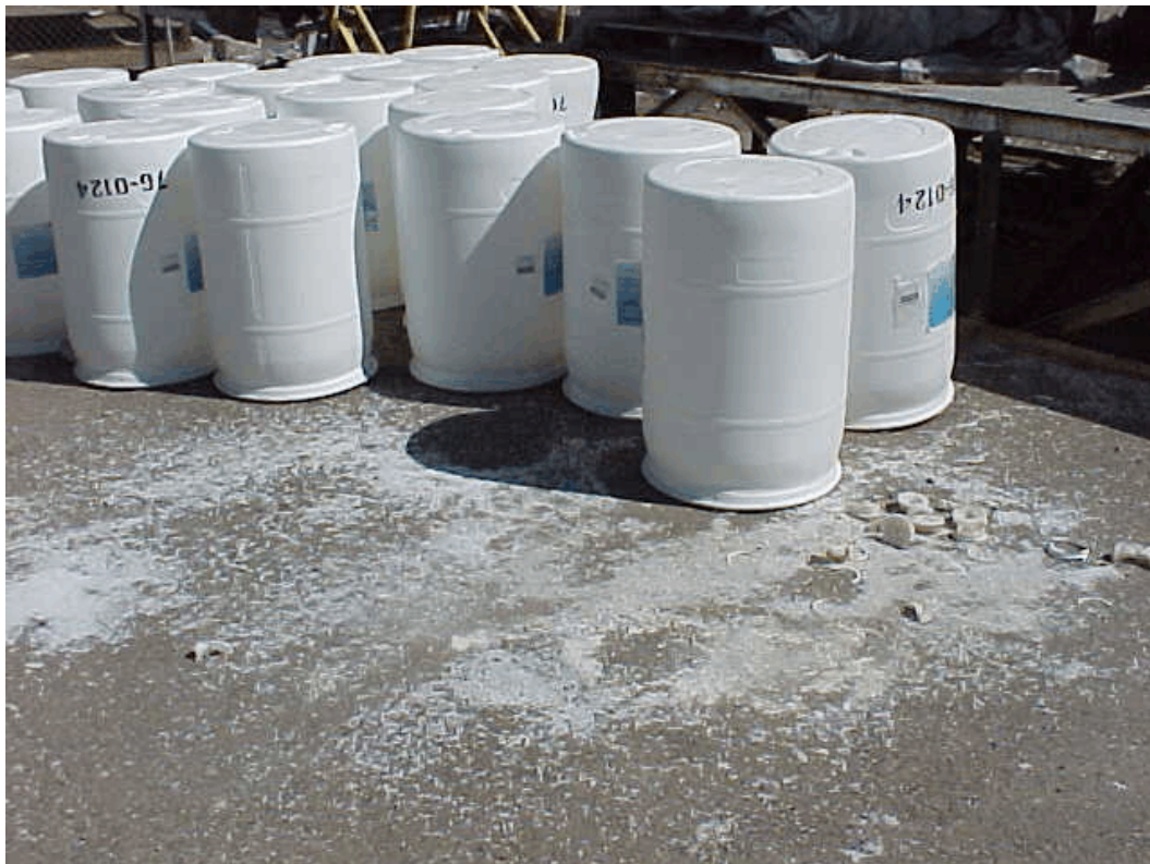
Photo 20. Vector Control facility: Empty drums of larvicide had been cut open in an uncontained location and residue spilled to the pavement.
