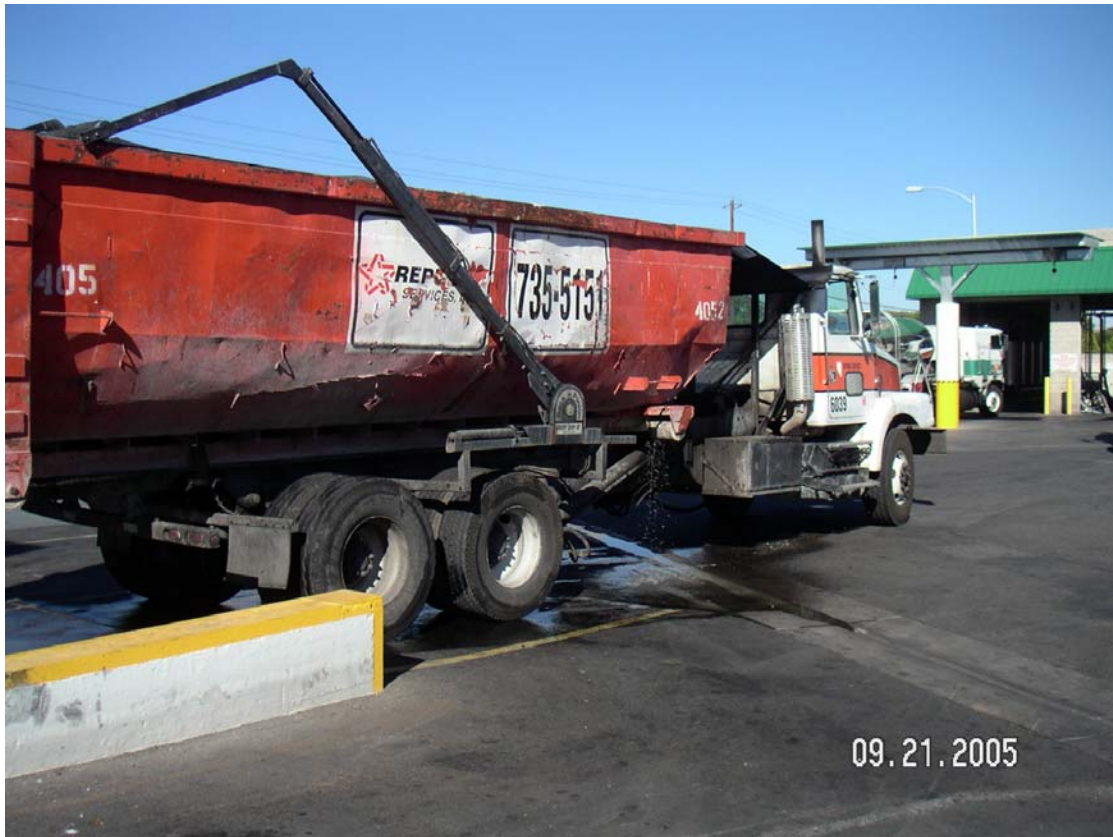
Photo 3. Roll-off container is leaking.
