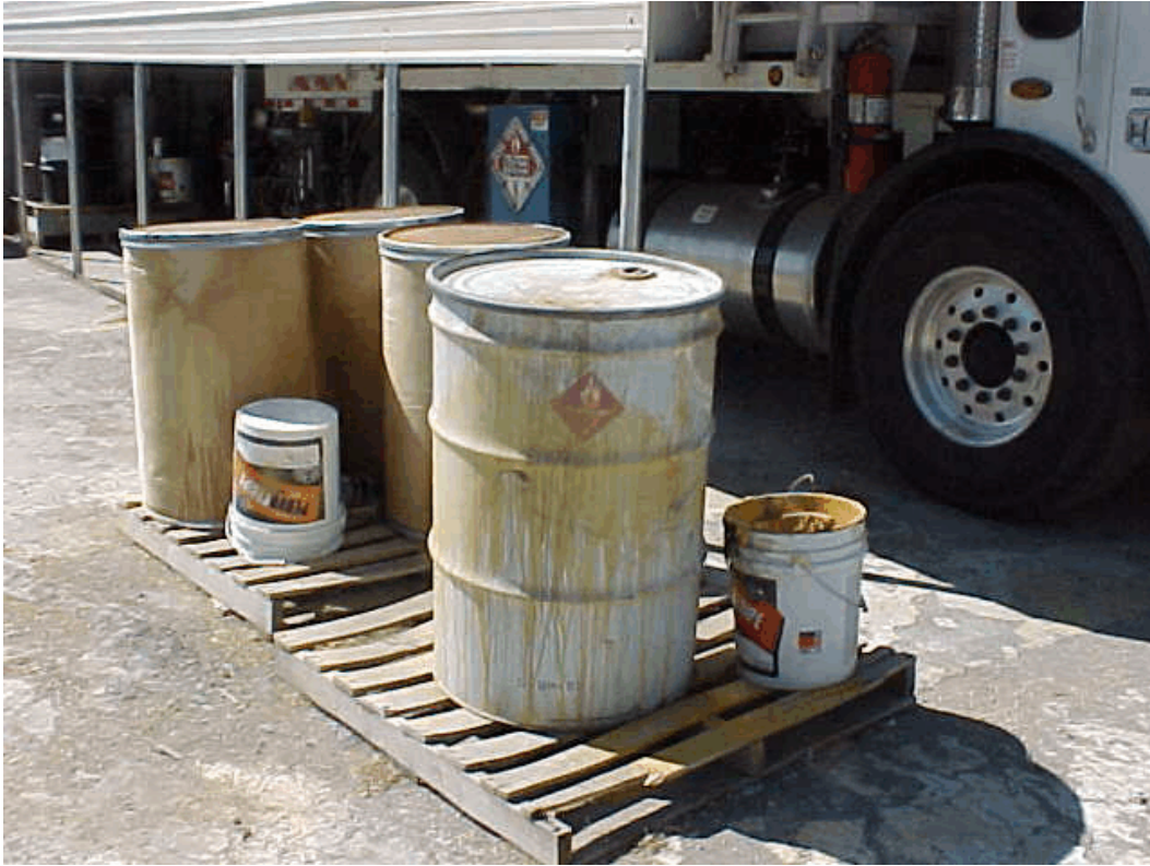
Photo 21. Traffic facility: One 55-gallon drum of flammable contents and three fiber drums of unknown contents were uncovered and uncontained.
