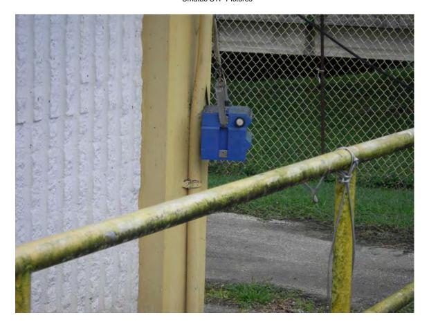
Picture 4: Data logger storing depth measurements.
