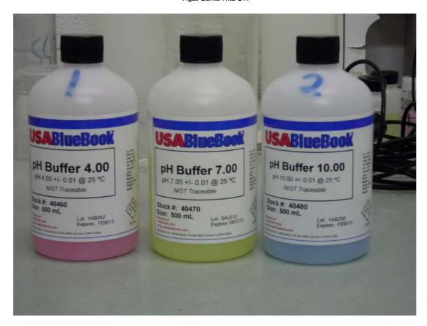
Picture 27: pH buffers used for calibration.
