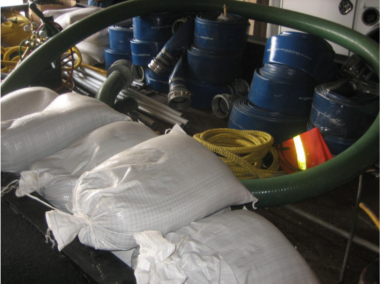
Figure 3: Spill response trailer with sandbags used for spill containment
