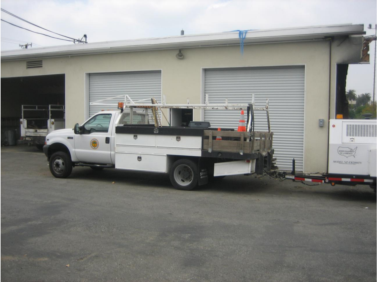
Figure 5: Utility truck with generator/jet rodder/CCTV trailer
