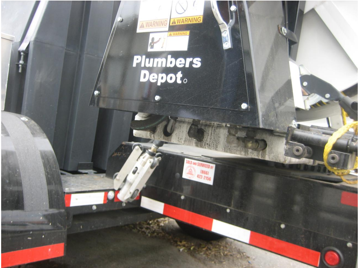
Figure 9: CCTV head on the generator/jet rodder/CCTV trailer
