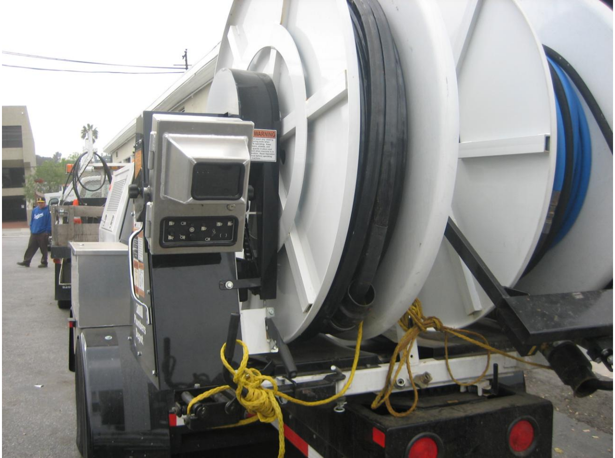
Figure 7: CCTV cable reel on trailer
