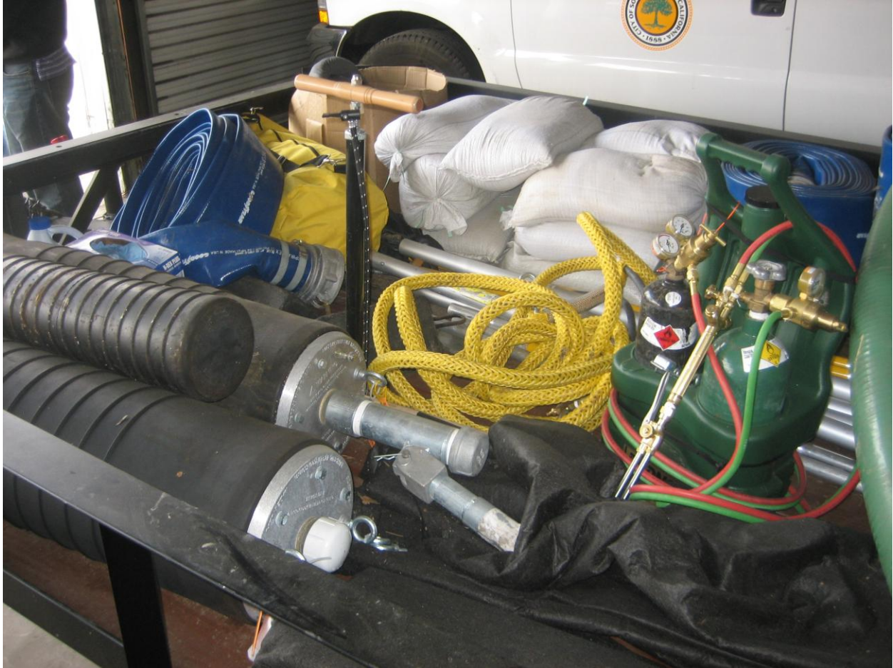
Figure 4: Spill response trailer with plugs, hoses, and sandbags
