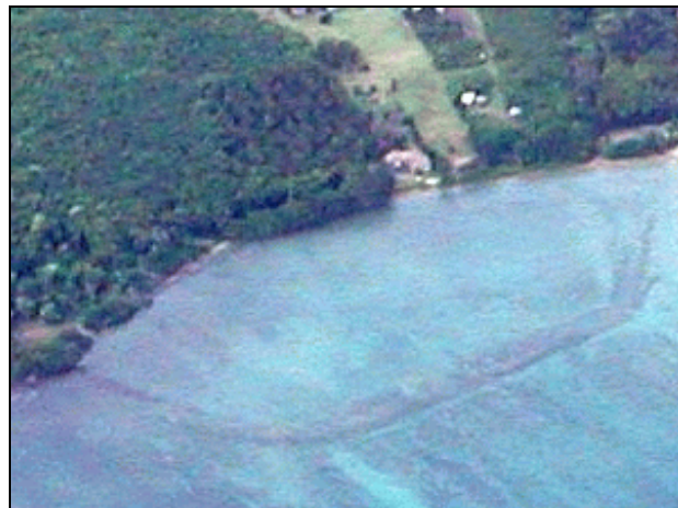
Figures 31, 32. No two fishponds are alike. Niaupala Fishpond (control pond) above right , and Panahaha Fishpond, left . Two fishponds with very different water circulation dynamics. Note Niaupala is actually an enclosed bay; Panahaha's wall was built out onto the reef resulting in better water circulation and water quality.
