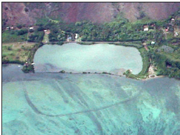
Figures 31, 32. No two fishponds are alike. Niaupala Fishpond (control pond) above right , and Panahaha Fishpond, left . Two fishponds with very different water circulation dynamics. Note Niaupala is actually an enclosed bay; Panahaha's wall was built out onto the reef resulting in better water circulation and water quality.
