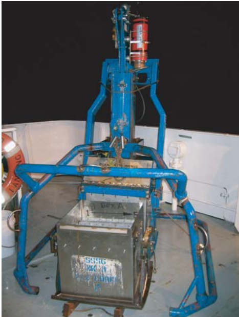
The 0.25 m 2 Sandia MK-III box corer
