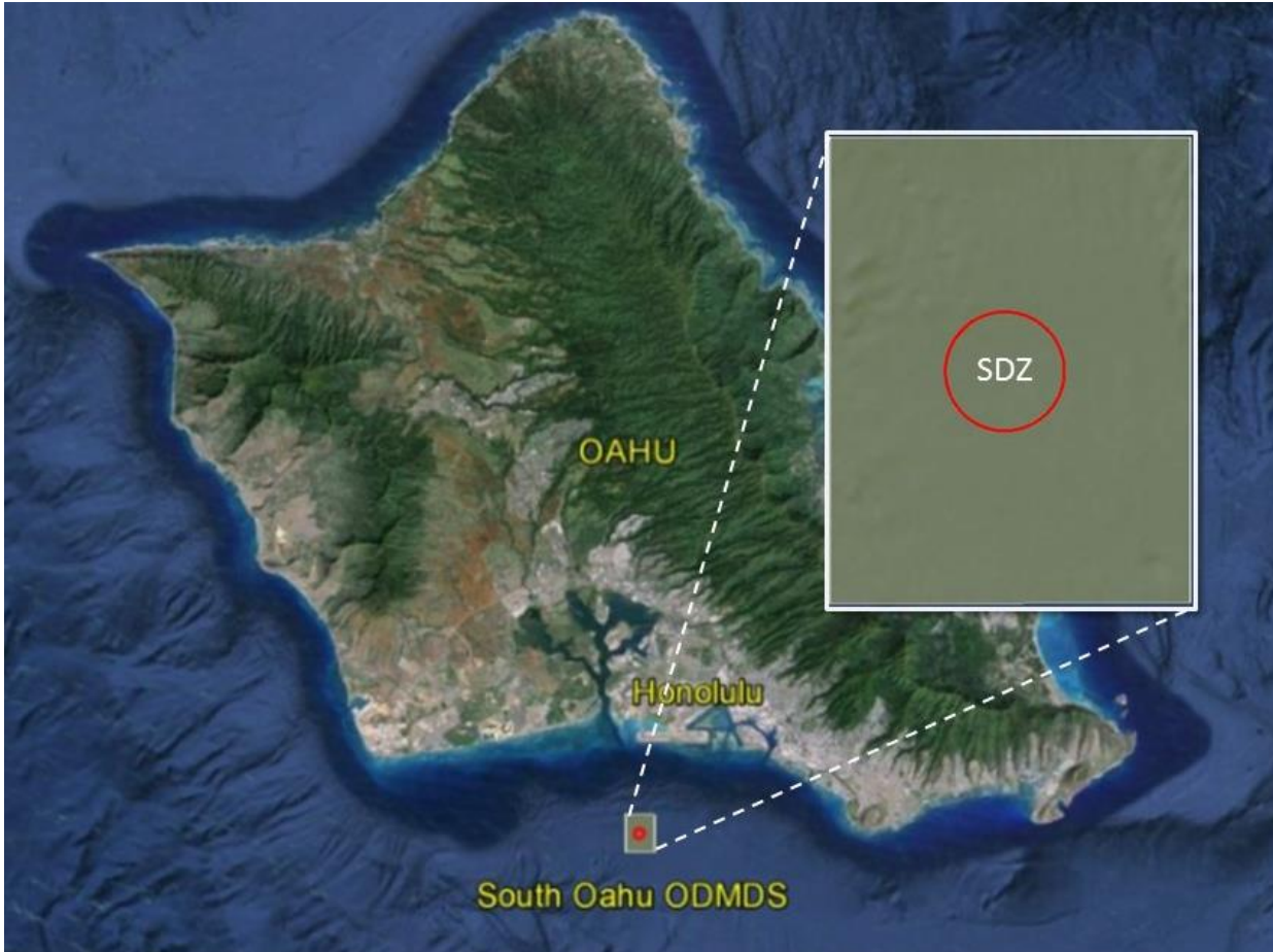
Figure 3. The South Oahu ODMDS, offshore of Honolulu, Oahu, Hawaii. White box is the site boundary on the seafloor; red circle is the Surface Disposal Zone (SDZ). All disposal operations must occur inside the SDZ unless specified otherwise in permits. Site coordinates and dimensions are shown in Table 1.
