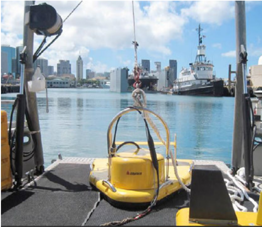
Figure 13. Sub-bottom profiler equipment – used only at the South Oahu site.
