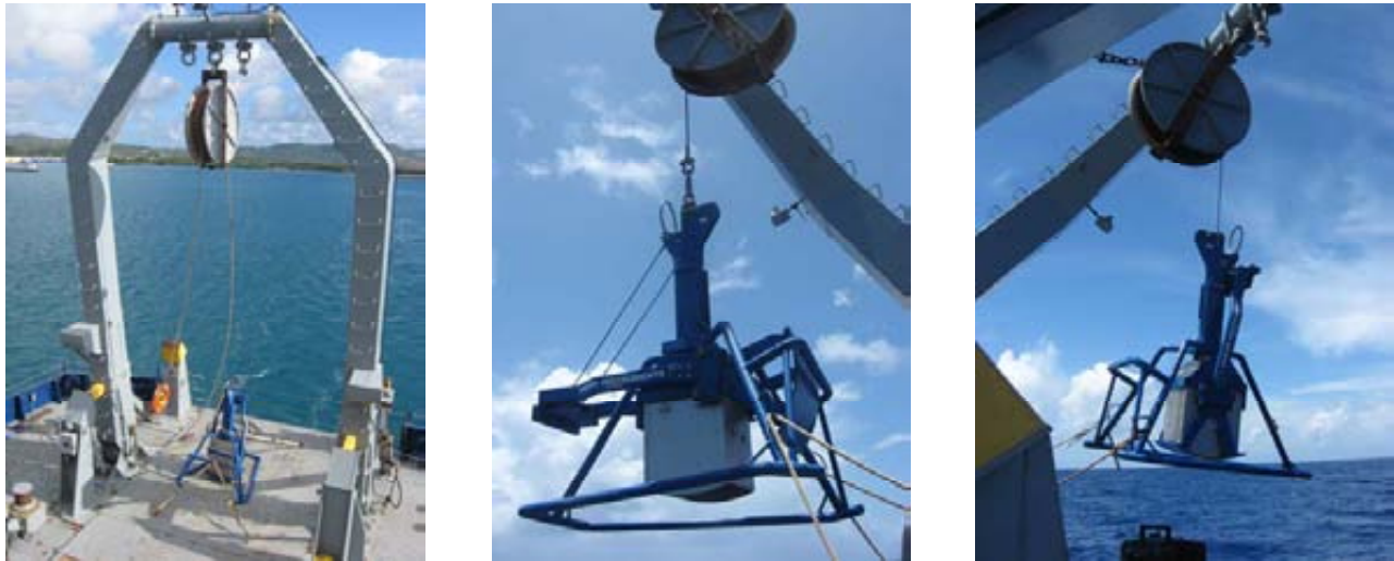
Figure 4. Sediment Sampling Equipment: Stern Mounted A-Frame Onboard the R/V Melville (left), Boxcore Being Deployed (center), Boxcore Being Retrieved (i.e. Triggered; right)
