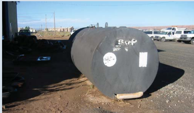
Steel tank with sacrificial anode (bottom) as corrosion protection.
