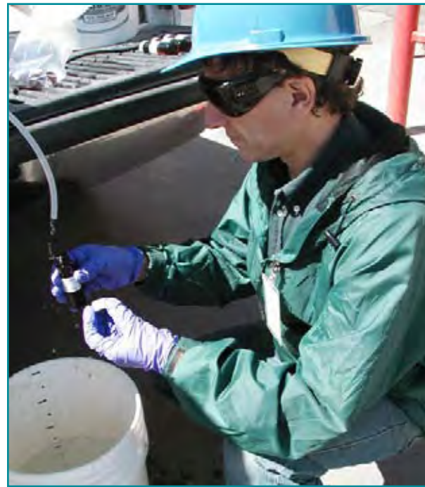
U.S. EPA Project Manager Ron Leach collecting a ground water sample.
