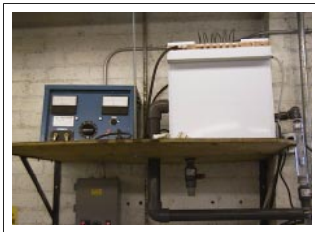
Figure 1. Electrowinning Rectifier and Electrolytic Cell
