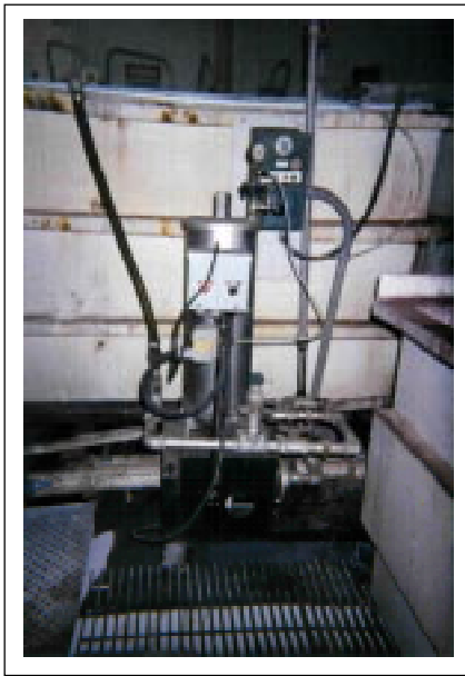
Figure 2. Nickel Acetate Bath Filtration System
