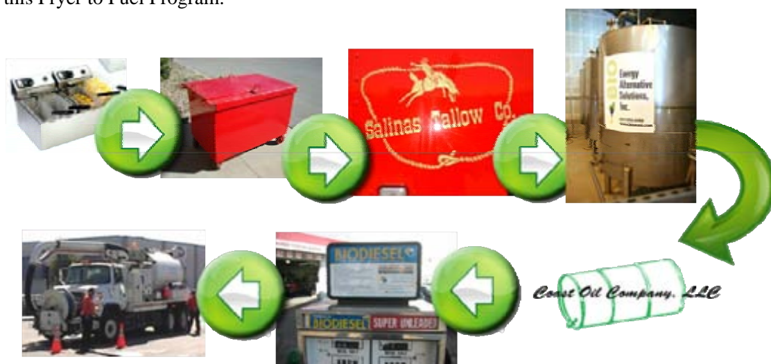
Figure 7. Fryer to Fuel Model: Oil goes from fryer to exterior bin, picked up by Salinas Tallow and treated, then taken to EASi to make into biodiesel, then to Coast Oil for blending and distribution, then to storage tanks, and then fuel for public fleets.
