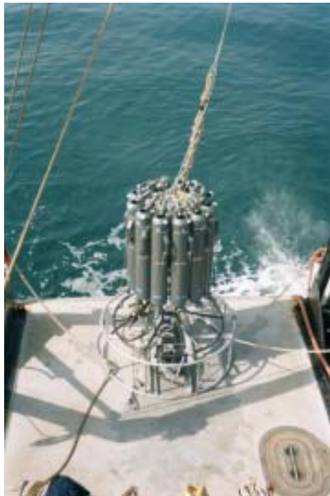
Figure 3-21. Rosette sampler used to collect water samples from plume and conductivity, temperature and depth (CTD) data
