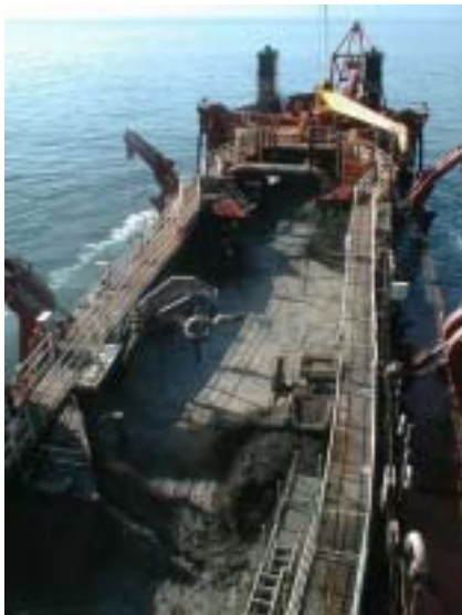
Figure 2-2. Photos of the hopper dredge Sugar Island , showing filling and cap placement operations
