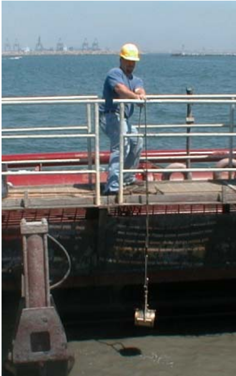
Figure 3-17. Retrieval of grab sample from hopper bin of dredge Sugar Island
