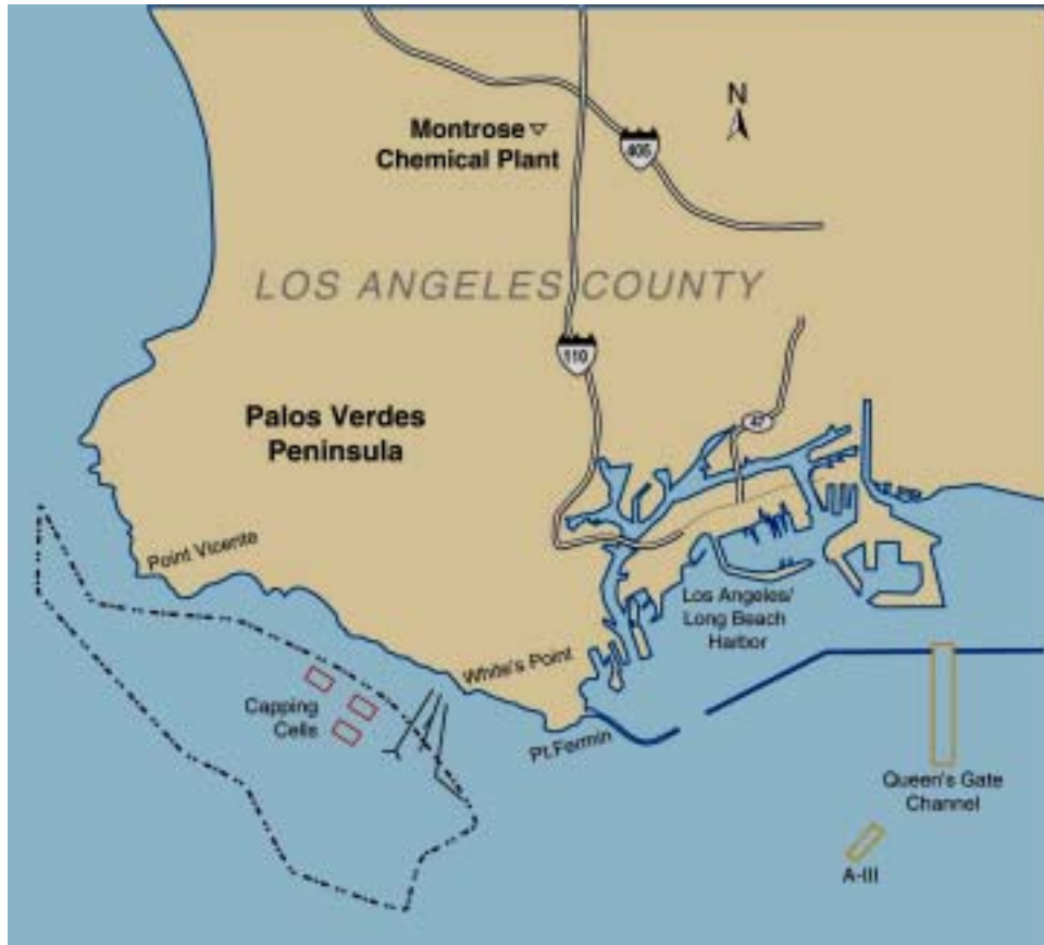
Figure 1-1. Location map showing Palos Verdes Shelf and slope, showing EA sediment footprint, pilot capping cells, Queen's Gate entrance channel, and borrow site A-III
