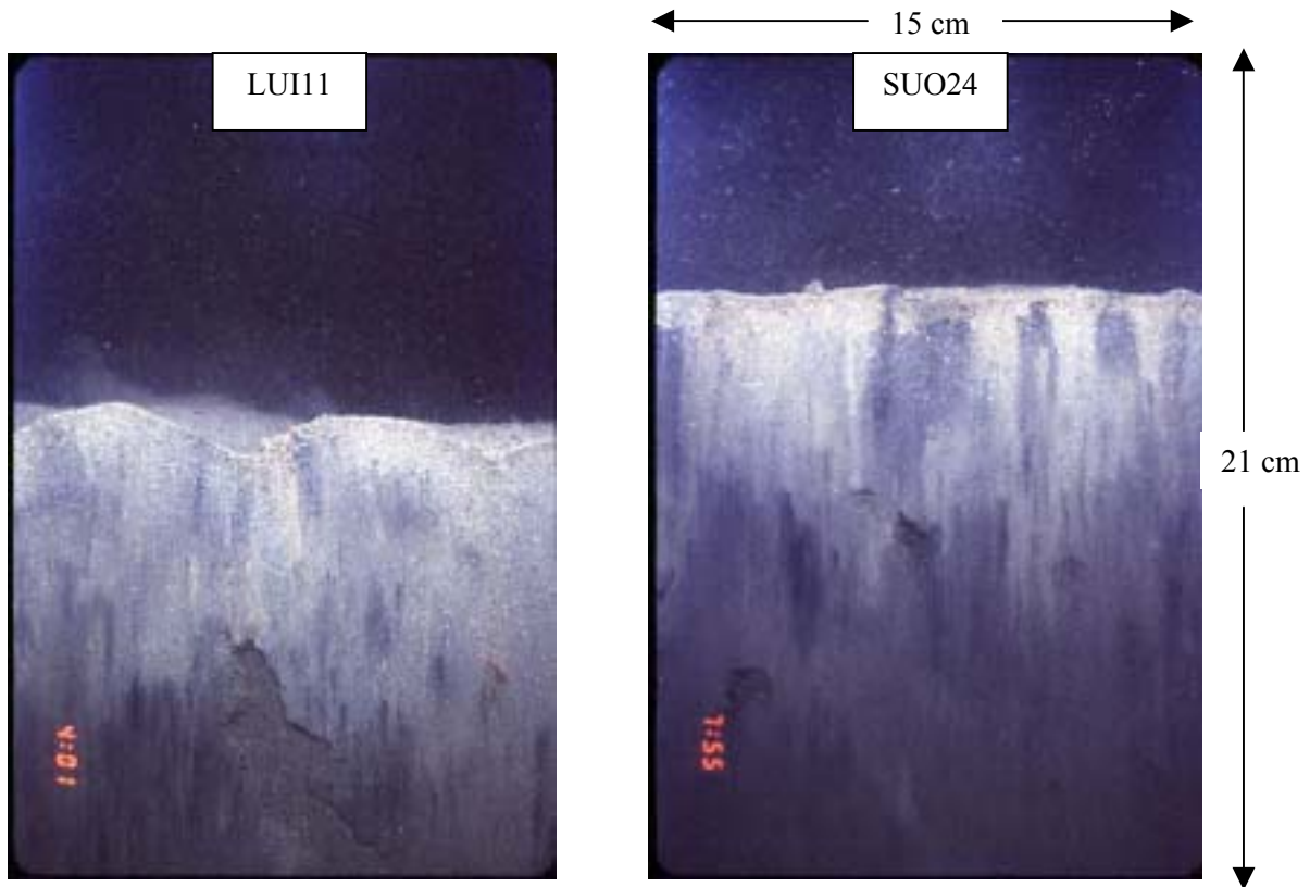
Figure 3-34. Comparison of representative SPI photos from landward (LUI11) and seaward cells (SUO24) showing difference in small scale topography resulting from biological burrowing activity
