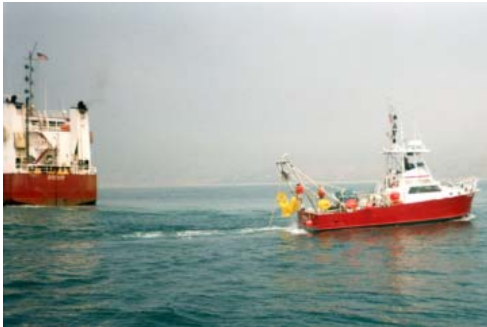
Figure 3-19. Deployment of drogue from MV Tuna in plume behind Sugar Island
