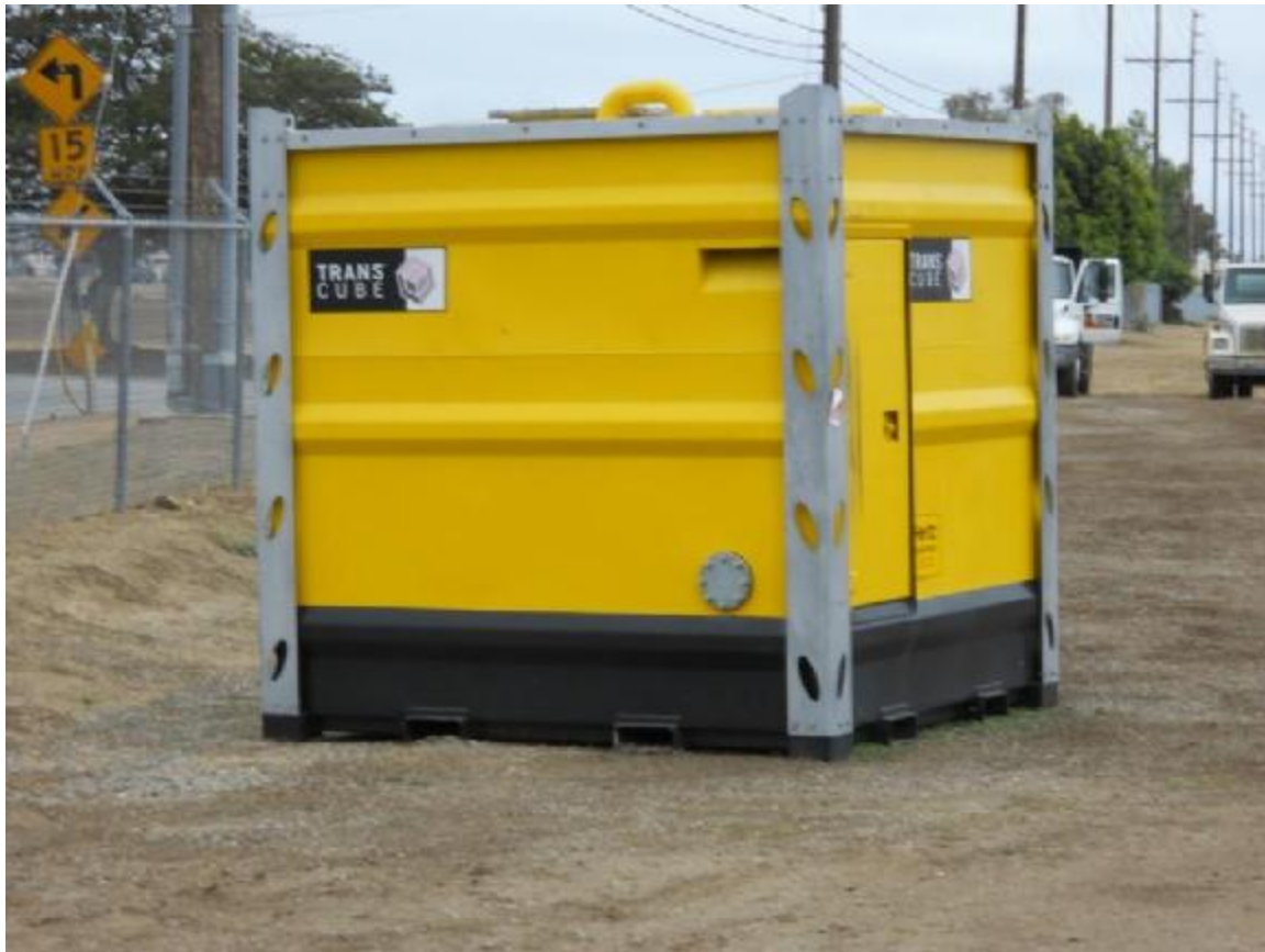
Figure 12: Portable storage container used to store fuel for diesel powered pumps during injection testing
