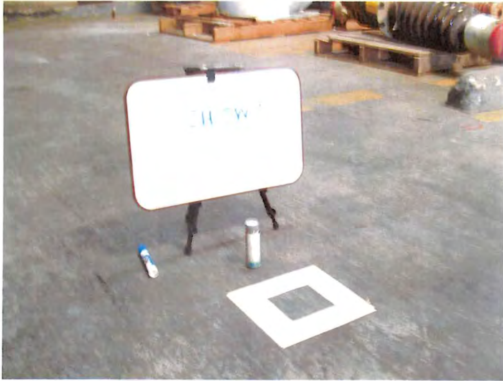
Photo 21 :View of wipe sample #5 collected inside PCB storage bay.
