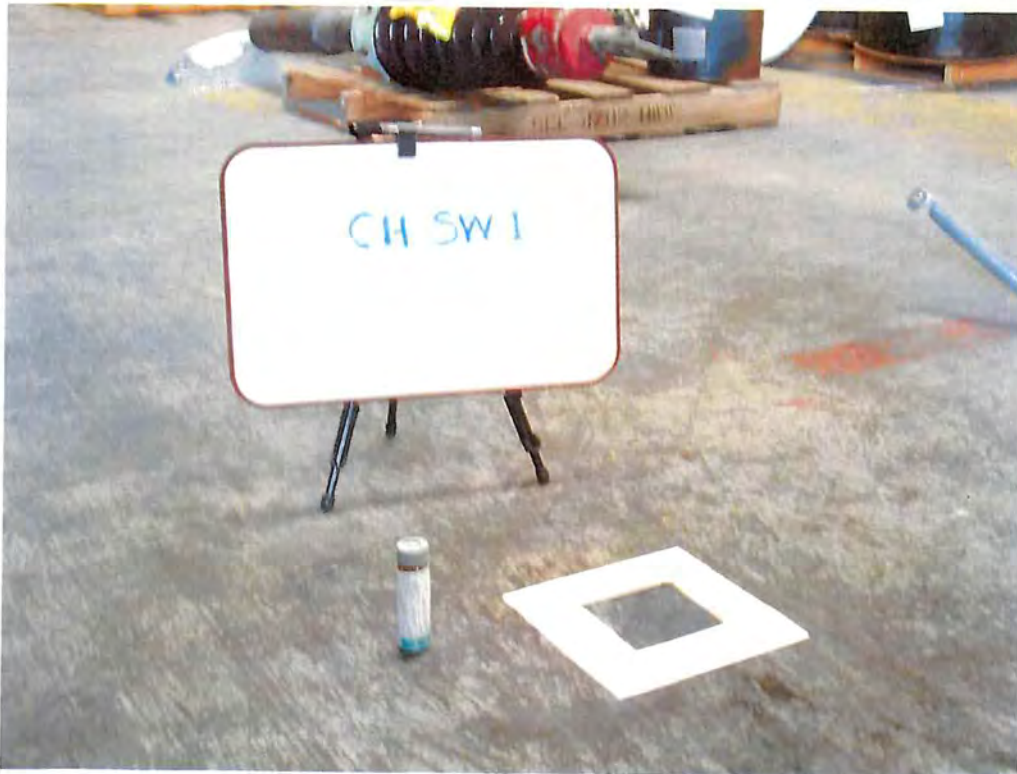
Photo 18 :View of wipe sample #1 collected inside PCB storage bay.
