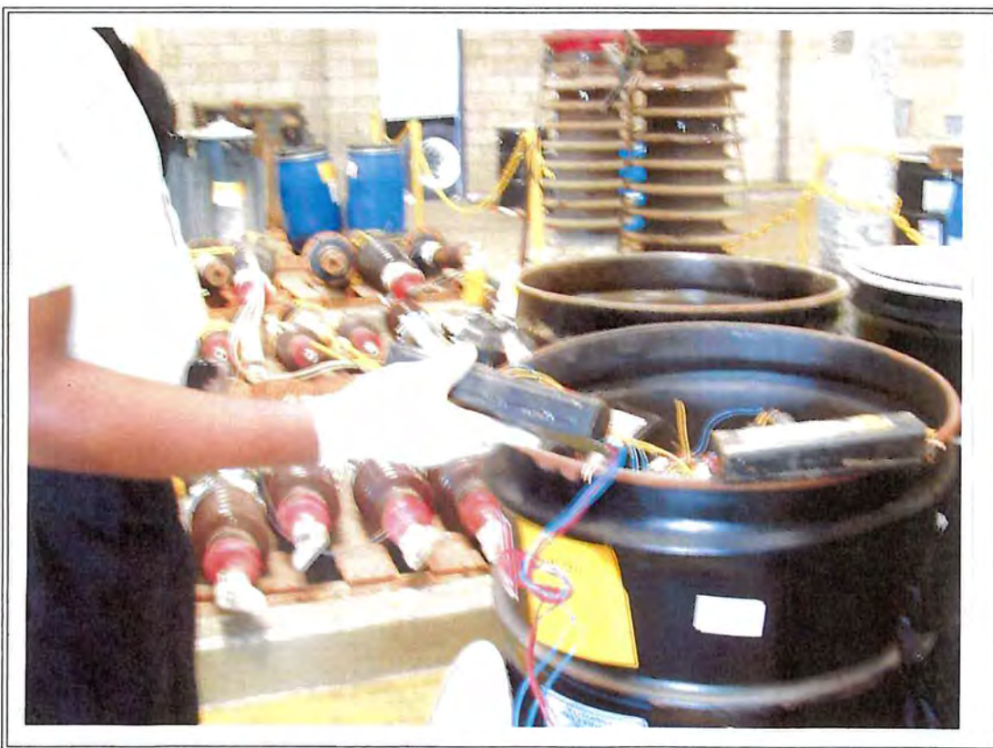
Photo 28 : Selecting ballast samples inside CHI "Container Storage Warehouse."
