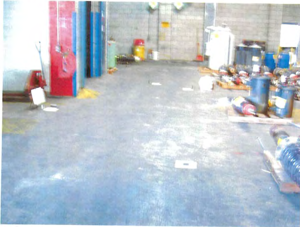
Photo 17 : Templates showing locations of wipe samples inside PCB storage bay in CHI's Container Storage Warehouse.
