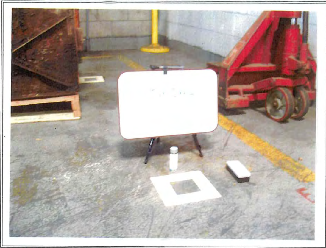
Photo 19 :View of wipe sample #2 collected inside PCB storage bay.
