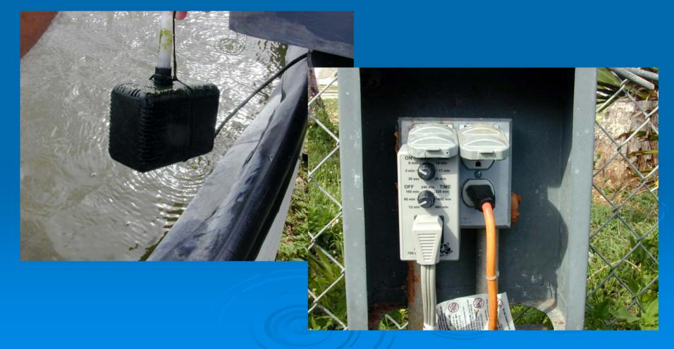
Timer allows plant tank to fill with water, then shuts off and drains back to fish tank.
