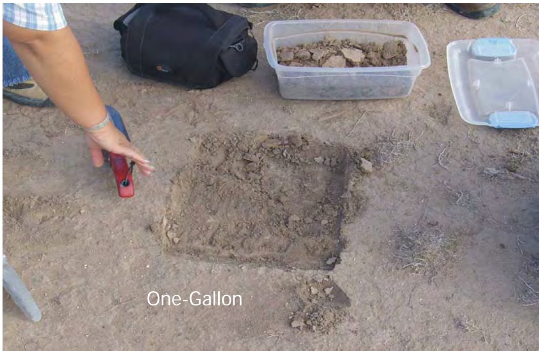
Figure 2-2. Collection of Arizona Soil One-Gallon Sample
