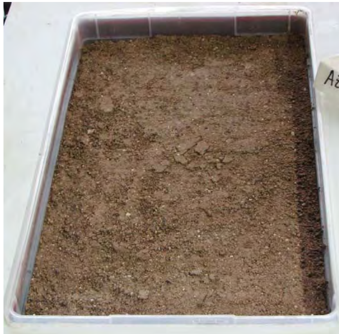
Figure 2-6. Typical AZ Soil Tray Before Product Application and Raking
