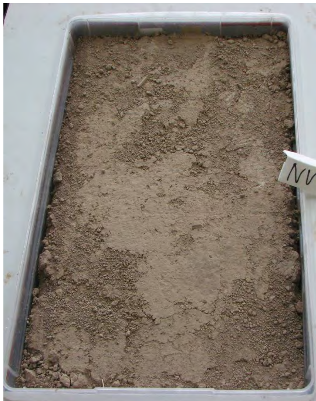
Figure 2-7. Typical NV Soil Tray Before Product Application and Raking
