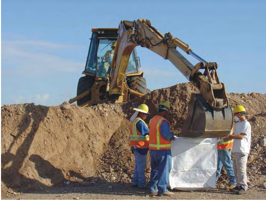
Figure 2-1. Collection of Arizona Soil Bulk Sample
