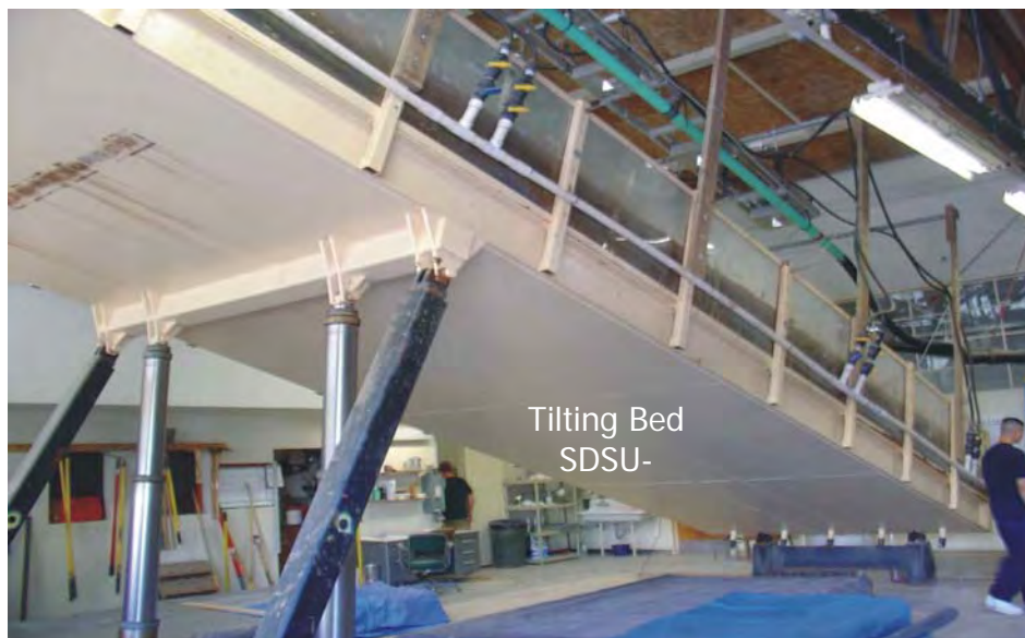
Figure 2-5. Tilting Test Bed (underside view)
