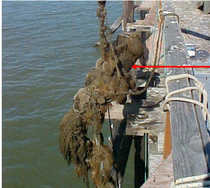
Figure 8-6: Marin Municipal Water District (MMWD) Seawater Desalination Pilot Program Intake after Three Months with No Cleaning from April to June 2006
