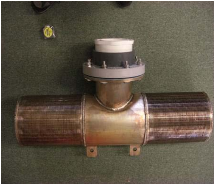
Figure ES-6: Pilot Scale Narrow-Slot Cylindrical Wedgewire Screen, (Tenera, 2010)
