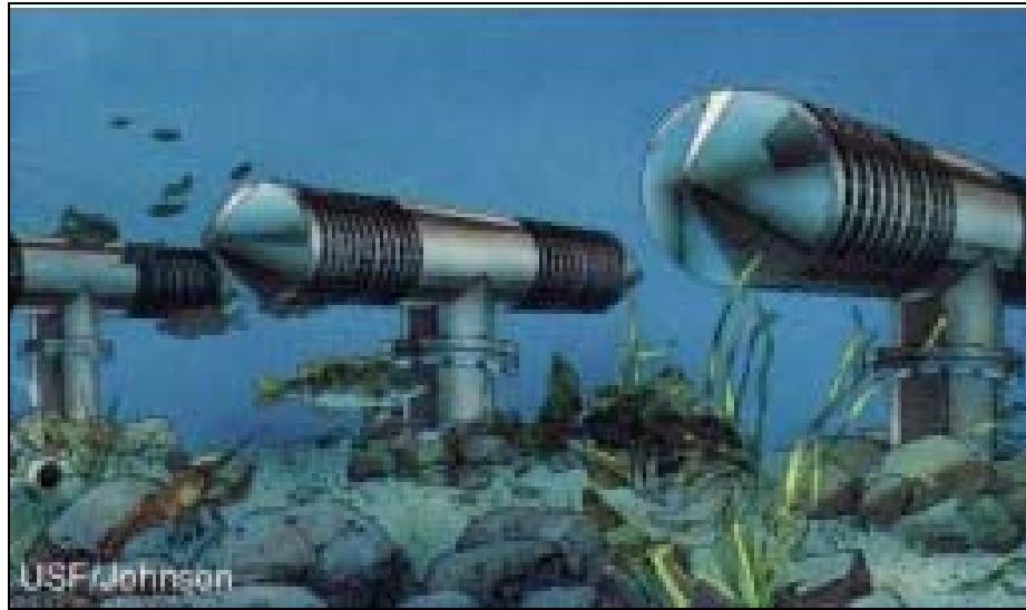
Figure 8-4: Rendering of an Offshore Cylindrical Wedgewire Screen Intake System (Tenera, 2010)
