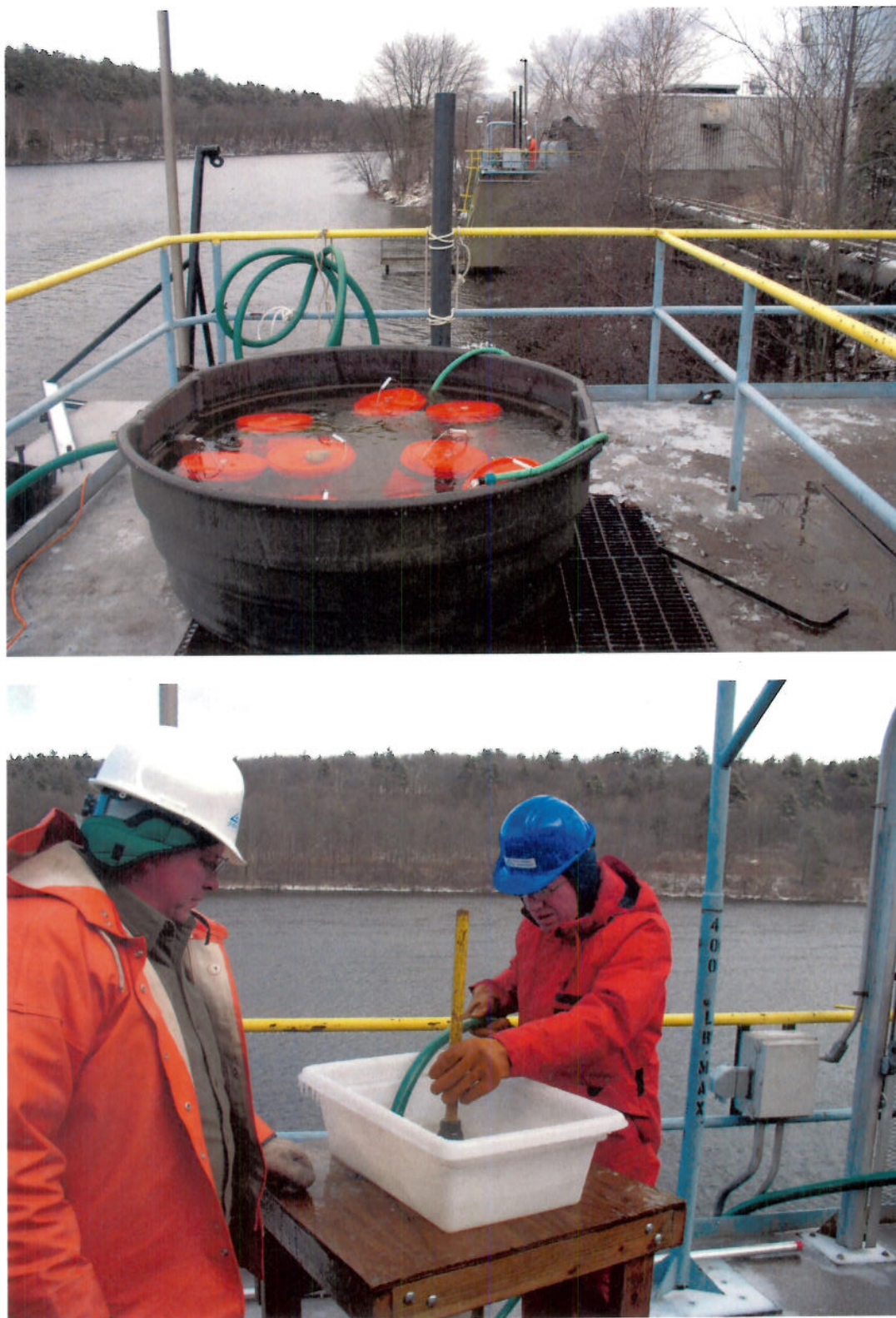
Figure 2-7. Injection device (bottom panel) and fish holding facility (upper panel) used at Units 1 and 2 of Merrimack Station for the release of fish onto the traveling screens associated with collection efficiency and impingement survival testing.
