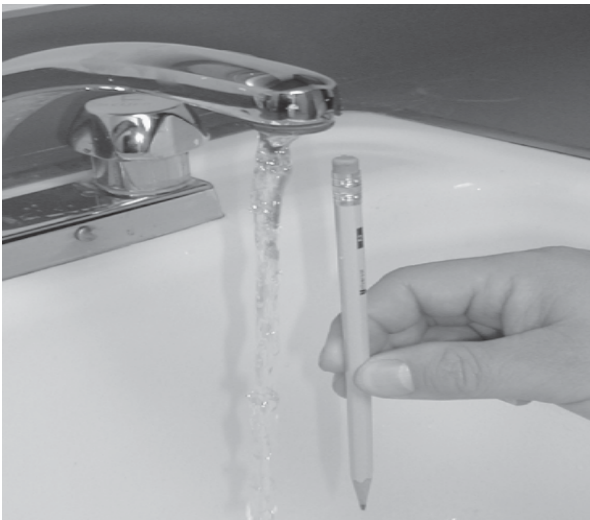
Adjusting the water to about a 1/4 inch diameter flow
