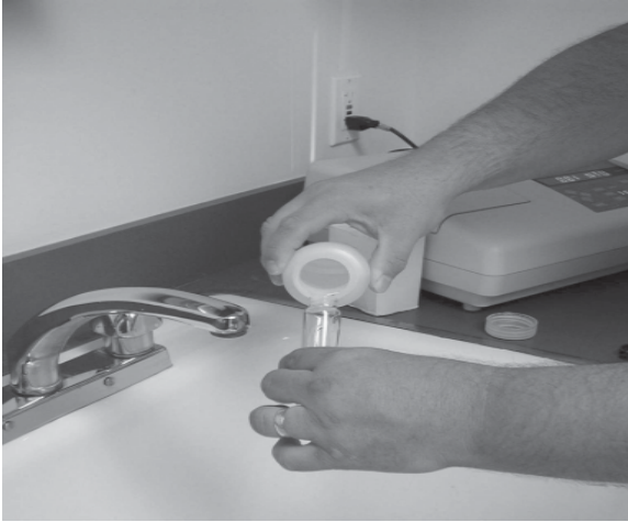
Transferring the sample to a glass sample tube
