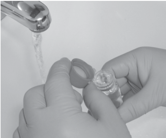
Topping off the vial with the bottle cap to form a meniscus
