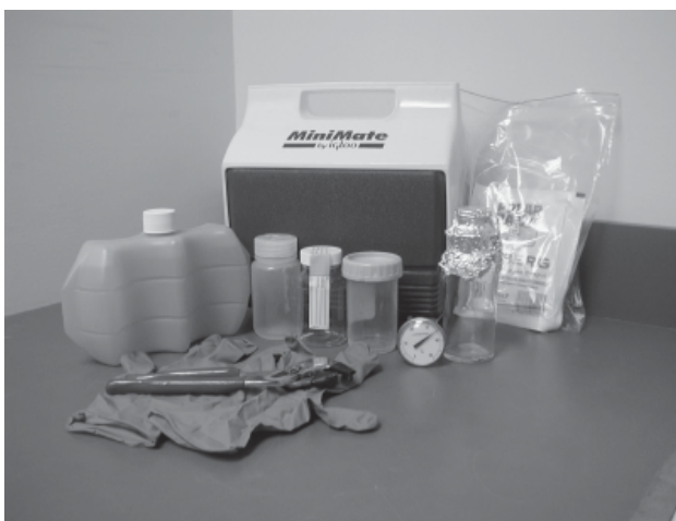
Typical sampling containers and equipment used for coliform sampling
