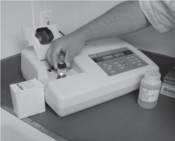
Calibrating the turbidimeter according to manufacturer's instructions
