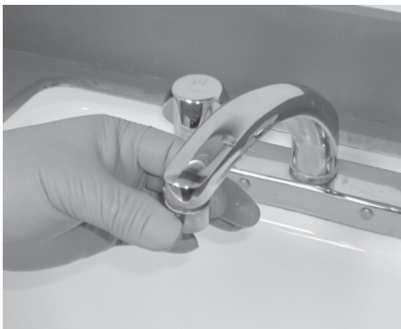
Removing aerator from faucet before starting to sample
