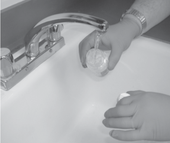
Holding the bottle under the water flow with cap in other hand
