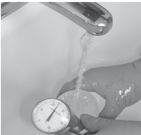
Flushing the tap until the water temperature stabilizes
