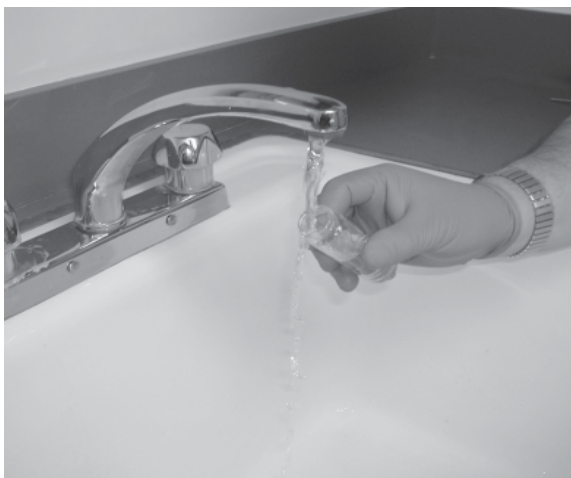
Tilting the vial to prevent formation of air bubbles
