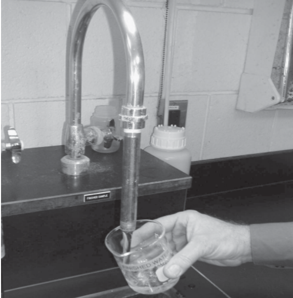
Collecting the sample from finished plant effluent
