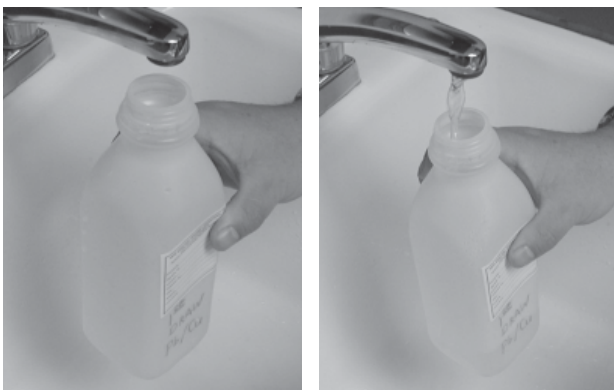
Holding bottle under the tap (left) before turning on the water (right)
