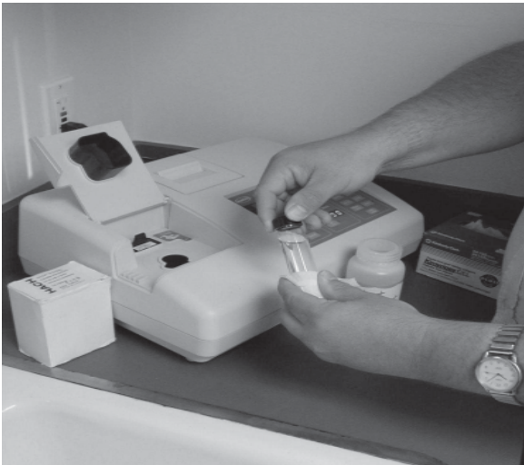
Wiping the outside of the tube
