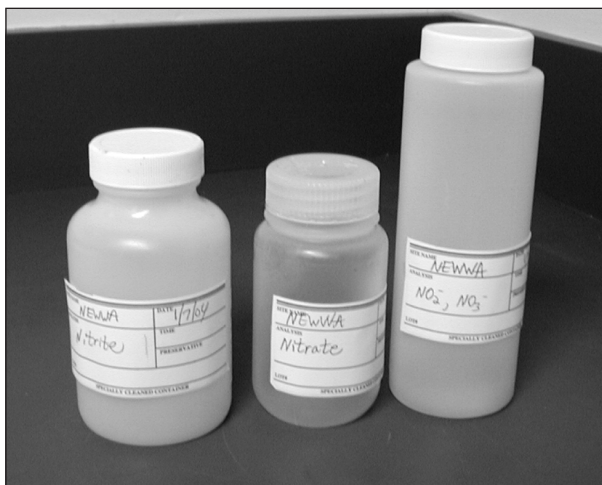
Typical nitrite and nitrate sampling containers.
