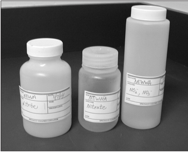
Typical nitrite and nitrate sampling containers.
