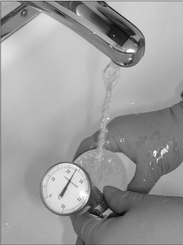
Flushing the tap until the water temperature stabilizes.
