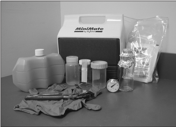
Typical sampling containers and equipment used for coliform sampling.
