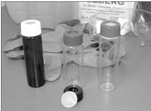
Typical VOC sampling containers and equipment.
