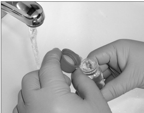
Topping off the vial with the bottle cap to form a meniscus.
