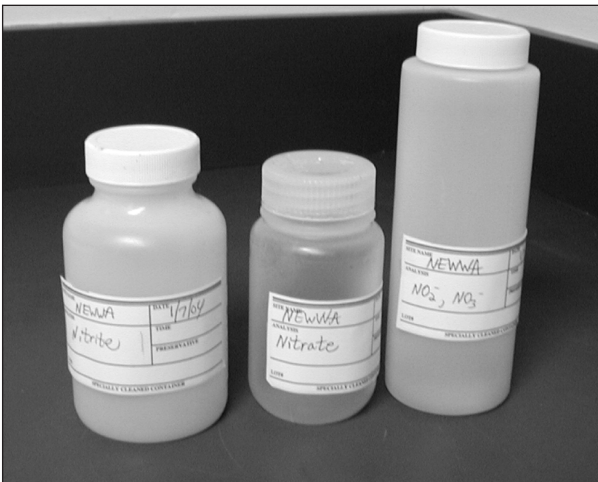
Typical nitrite and nitrate sampling containers.
