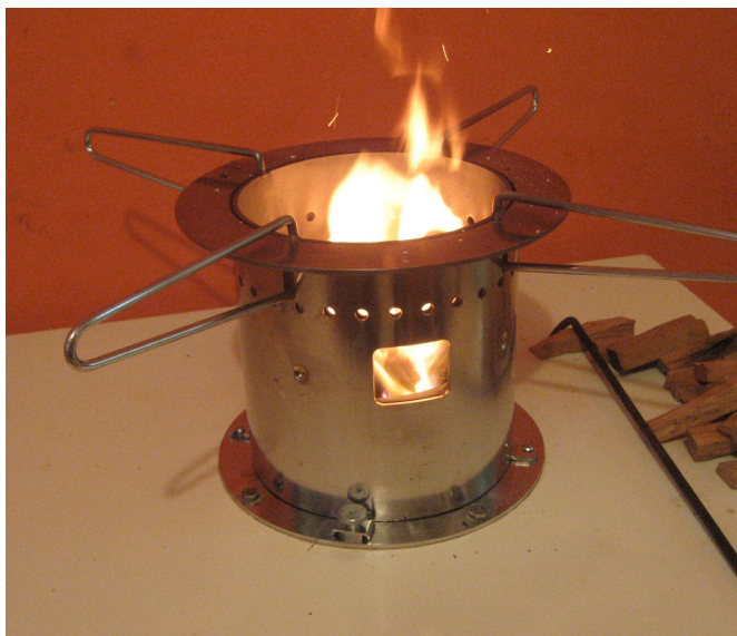
Figure 10-4. The Turbococina Stove , which burns wood, is made of a stainless steel cylinder fitted with 10 air injectors, an internal fan that runs on electricity, and a steel plate that regulates the air flow to improve combustion efficiency. This stove is currently available primarily for institutional settings. (Photo courtesy of René Nuñez Suárez, Turbococina)
