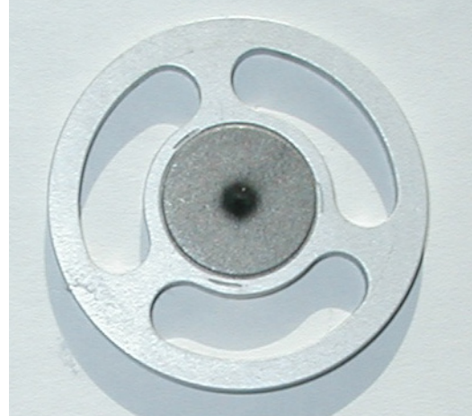
Figure 2-6. Coarse Urban PM (Diameter > 2.5 microns) with a Black Surface Coating, shown on a Filter from a Harvard Impactor Run Approximately 100 feet Above Street Level in Boston. (Photo courtesy of NESCAUM)
