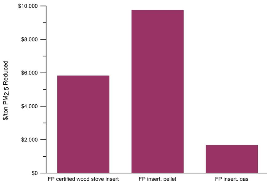
Figure 10-3. Cost Per Ton PM<sub>2.5</sub> Reduced (\$/Ton) for the Addition of an Insert into a Fireplace (2010\$). (Source: U.S. EPA, data courtesy of MARAMA)
