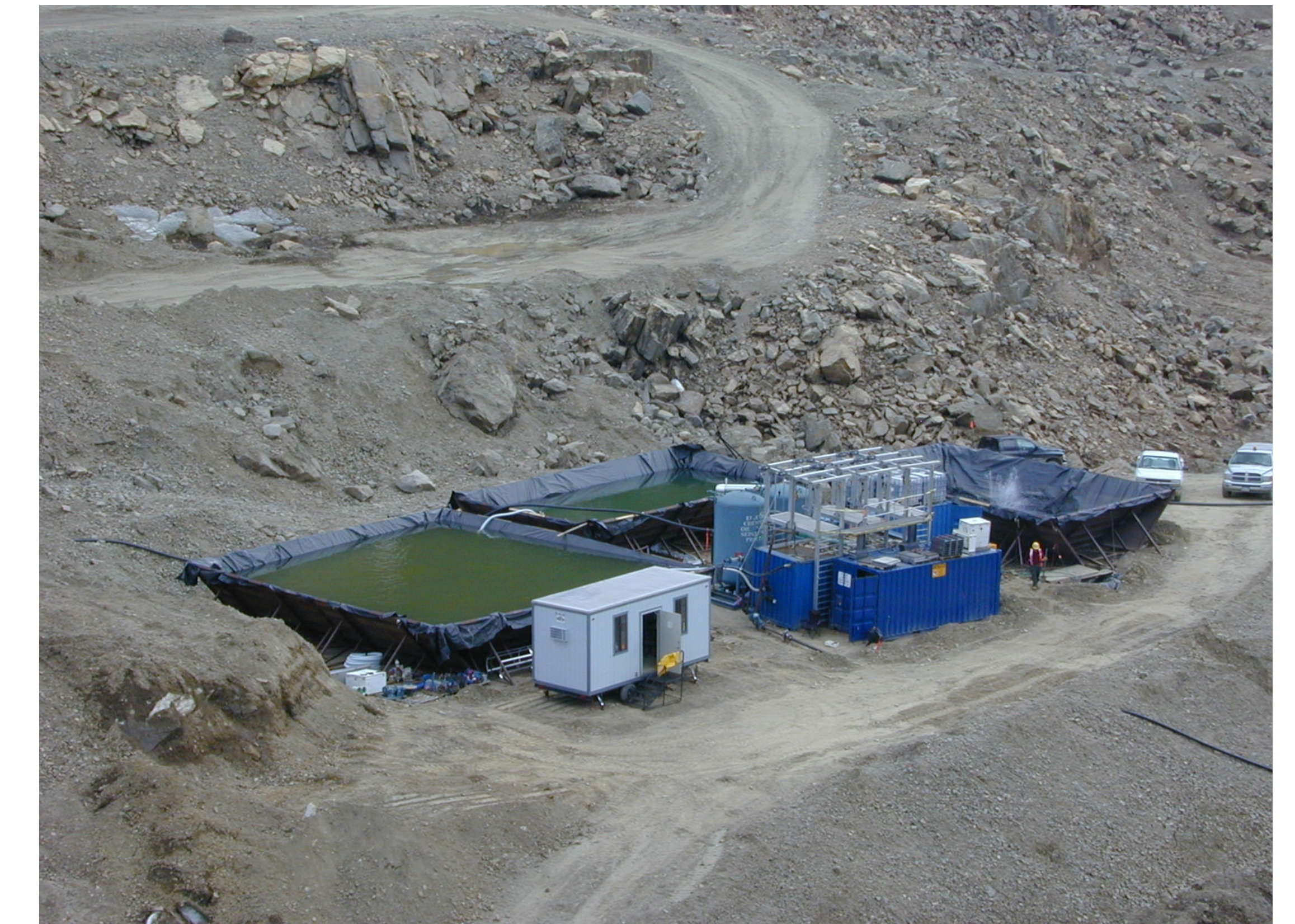
Figure 1: The above picture was taken of an electrocoagulation system that was being used in a dam resurfacing project in Colorado.
