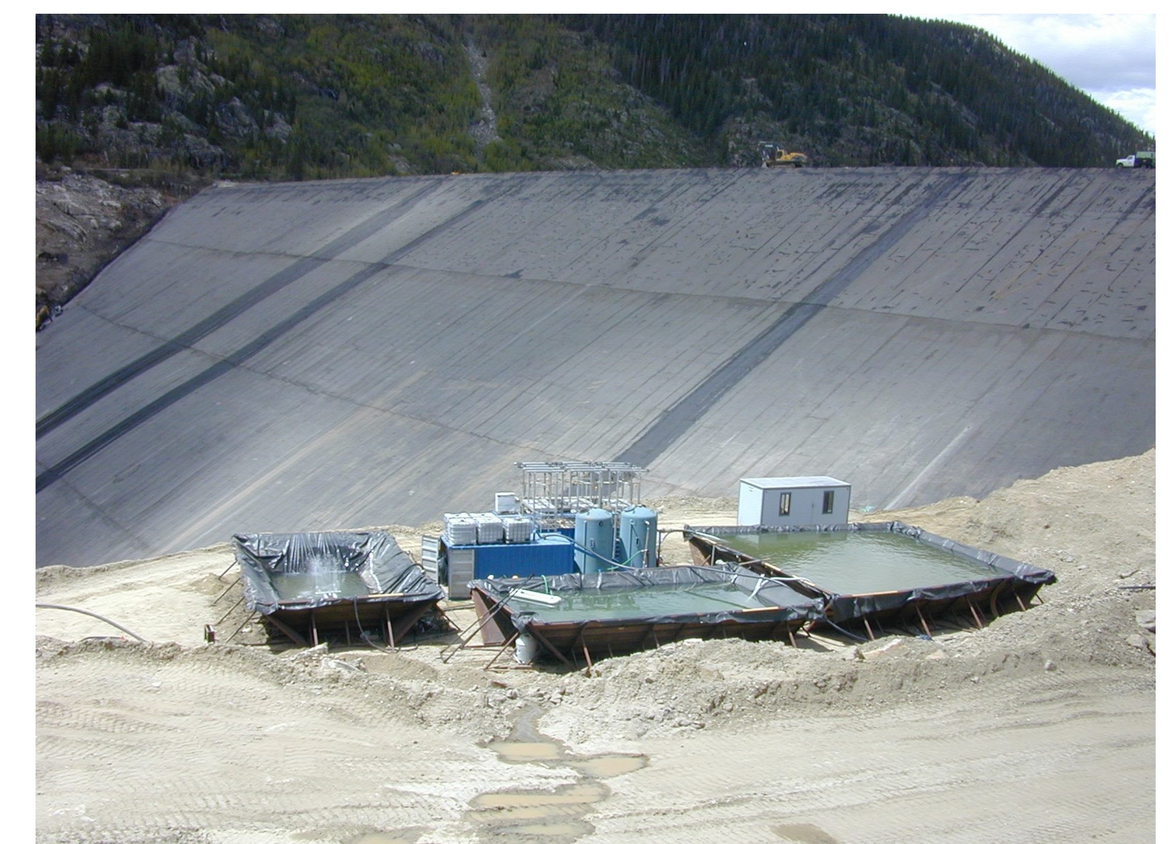
Figure 2: The electrocoagulation system can be set up in remote areas or incorporated into an existing process.
