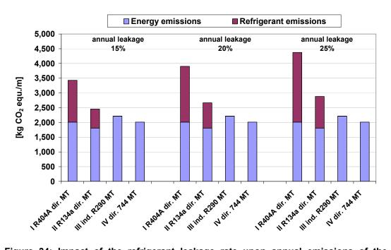
Figure 34: Impact of the refrigerant leakage rate upon annual emissions of the model technologies at the discounter
