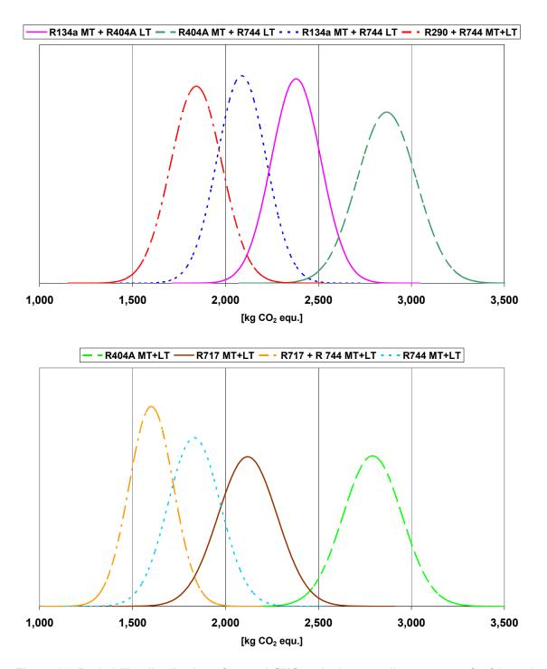
Figure 13: Probability distribution of annual GHG emissions per linear meter of refrigeration unit for supermarkets in connection with different layout options (leakage rate 11.65 %) (schematic)
