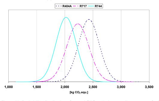
Figure 21: Probability distribution of annual GHG emissions per linear meter of refrigeration unit for the hypermarket in connection with different layout options (leakage rate 2.65 %) (schematic)
