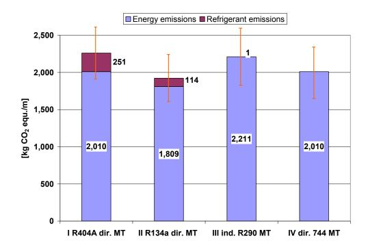
Figure 11: Annual GHG emissions per linear meter of refrigeration unit for the discounter in connection with different layout options (leakage rate 2.65 %)
