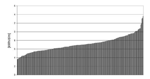
Figure 10: Daily normalised power consumption for refrigeration related to front meter of refrigerated cabinet in 226 Penny markets in 2001 [Ecofys2003].
