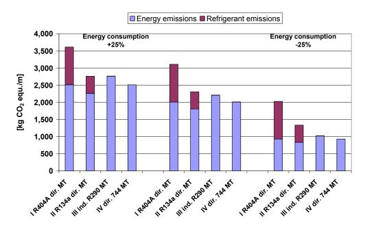
Figure 25: Impact of specific energy consumption upon annual greenhouse gas emissions of the model technologies used by the discounter (leakage rate 11.65%)
