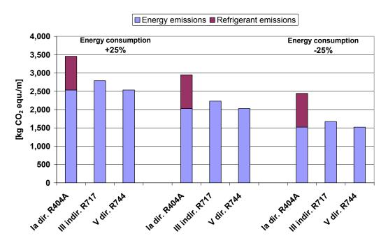
Figure 32: Impact of specific energy consumption upon annual greenhouse gas emissions of the model technologies used by the hypermarket (leakage rate 6.15%)
