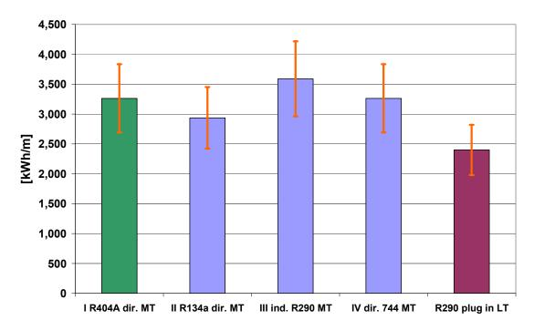
Figure 1: Annual energy consumption of the different refrigeration systems at the discounter
