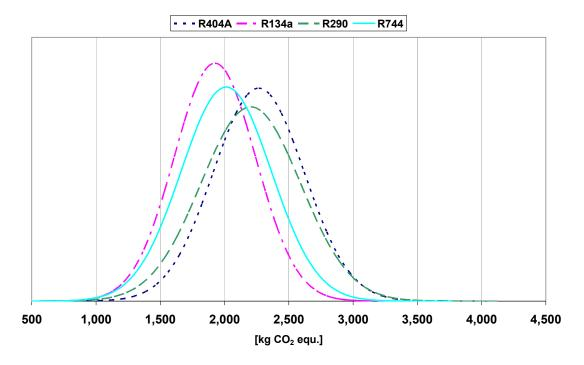
Figure 8: Probability distribution of annual GHG emissions per linear meter of refrigeration unit for the discounter in connection with different layout options (leakage rate 2.65 % = policy scenario 3) (schematic)
