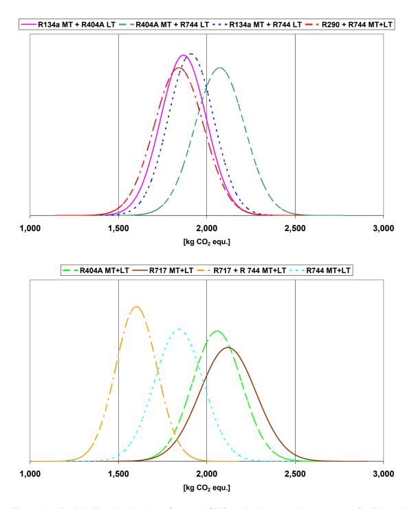
Figure 15: Probability distribution of annual GHG emissions per linear meter of refrigeration unit for supermarkets in connection with different layout options (leakage rate 2.65 %) (schematic)
