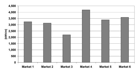
Figure 3: Measured energy consumption at hypermarkets – multi-plex refrigeration system with HFC (Source: Retail chain)
