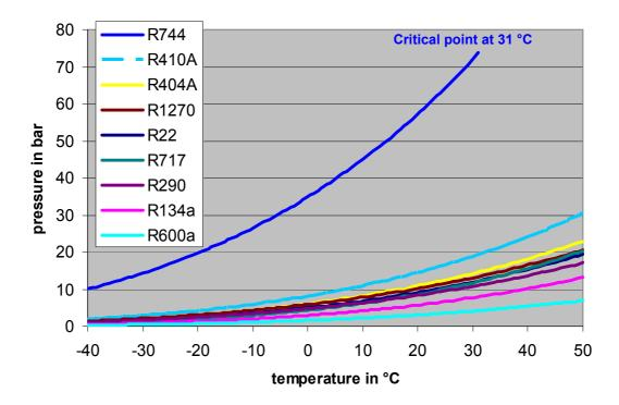
Figure 6: Vapor pressure curves of refrigerants used in supermarket refrigeration systems calculated with CoolPack version 1.46. In the caption, the refrigerants follow their vapor pressures, i.e. R744 with the highest evaporation pressure at given temperature on top and R600a with the lowest evaporation pressure at the same temperature at the bottom.
