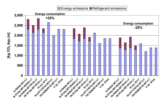
Figure 29: Impact of specific energy consumption upon annual greenhouse gas emissions of the model technologies used by the supermarket (leakage rate 6.15%)
