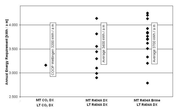
Figure 11: Energy need per front meter refrigeration unit in Swiss supermarkets.
