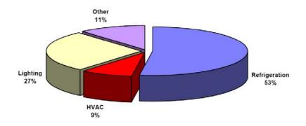
Figure 3: Energy consumption in a typical American supermarket with app. 4,650 m<sup>2</sup> and an energy consumption of 4.65 kWh/m<sup>2</sup> [Faramarzi2004].
