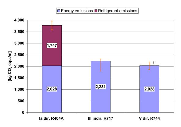
Figure 22: Annual GHG emissions per linear meter of refrigeration unit for the hypermarket in connection with different layout options (leakage rate 11.65 %)
