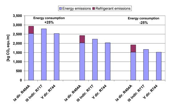
Figure 33: Impact of specific energy consumption upon annual greenhouse gas emissions of the model technologies used by the hypermarket (leakage rate 2.65%)
