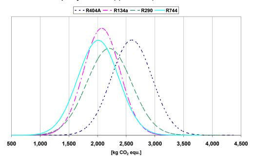
Figure 7: Probability distribution of annual GHG emissions per linear meter of refrigeration unit for the discounter in connection with different layout options (leakage rate 6.15 % = policy scenario 2) (schematic)
