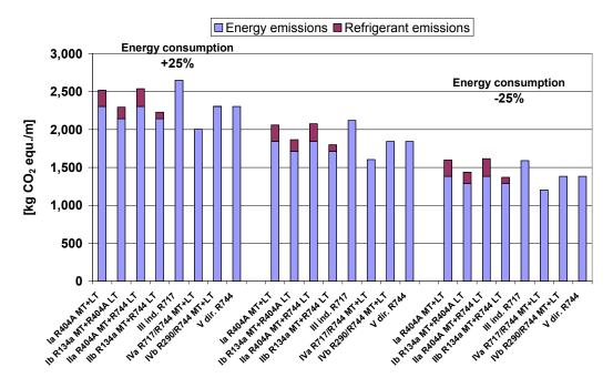
Figure 30: Impact of specific energy consumption upon annual greenhouse gas emissions of the model technologies used by the supermarket (leakage rate 2.65%)
