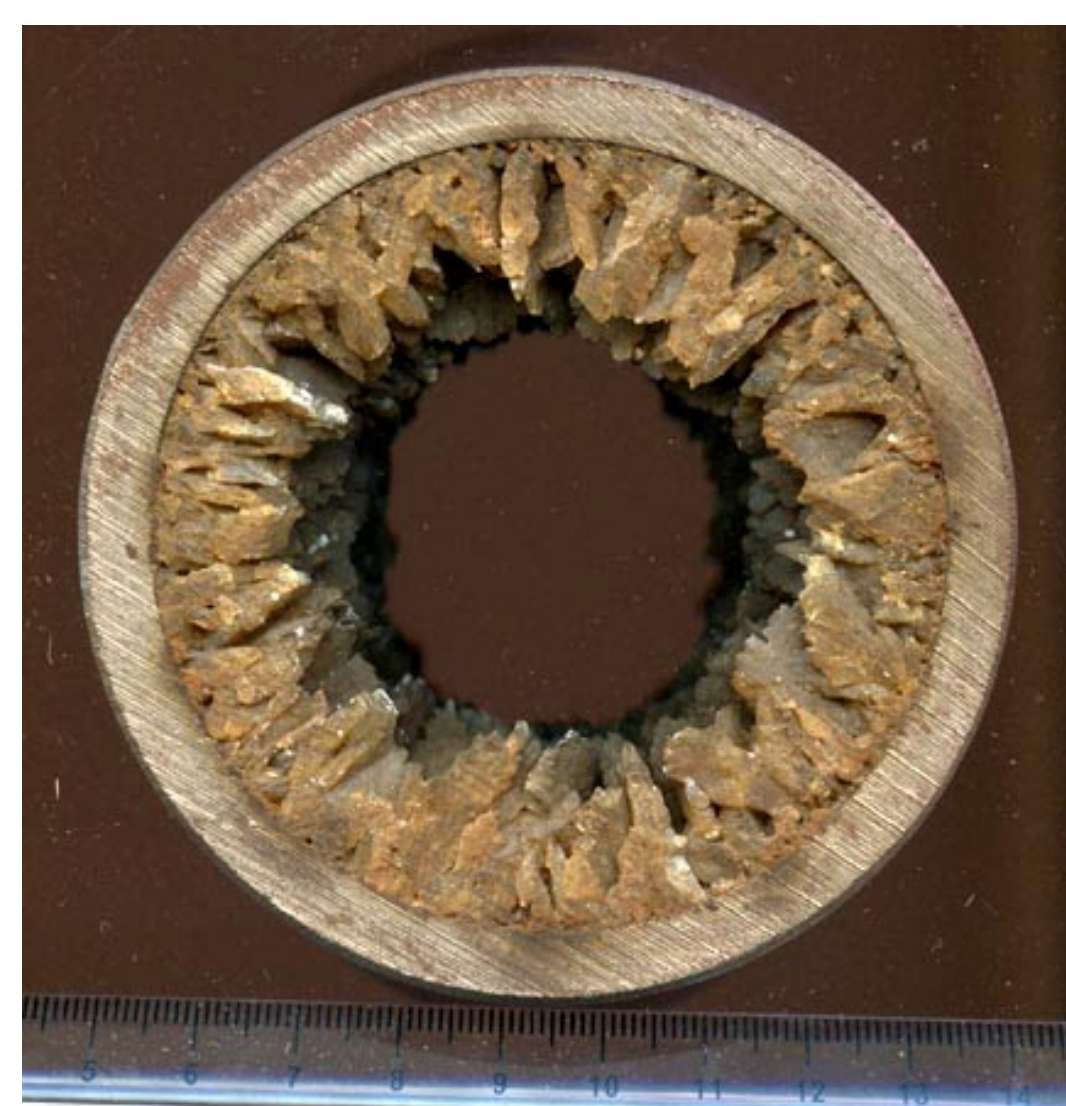
Figure 1. Barite scale in a pipe used to carry oil. ( http://theoildrum.com )
