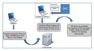
Figure 1: TRI-MEweb's transmission, certification and submission steps
