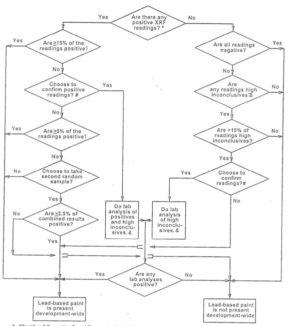
"Positive," "negative," and "inconclusive" XRF readings are determined in accordance with the XRF instrument's Performance Characteristics Sheet as described in the HUD Guidelines for the Evaluation and Control of Lead Hazards in Housing, chapter 7.
