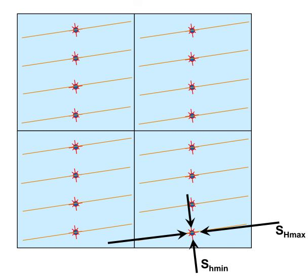
BH locations placed based on stresses in the earth which dictate hydraulic fracture orientation
