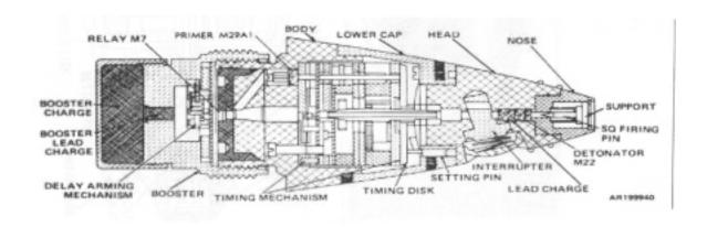
Figure 3-4. Mechanical Time Fuze
