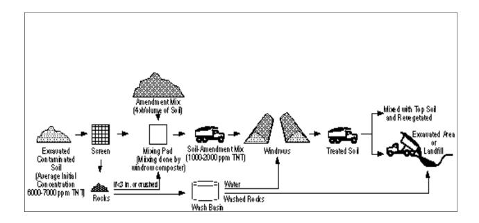
Figure 5-2. Typical Windrow Composting Process
