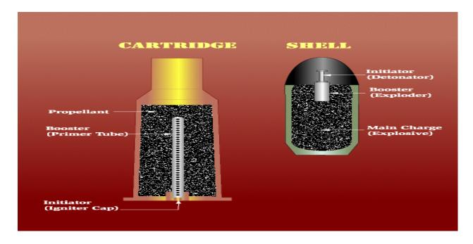
Figure 3-2. Explosive Trains in a Round of Artillery Ammunition
