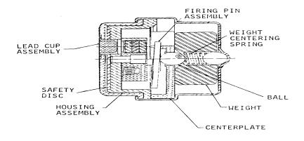
Figure 3-3. Mechanical All-Way-Acting Fuze
