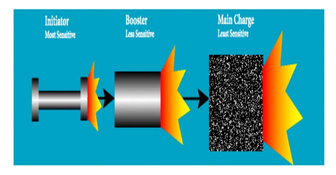
Figure 3-1. Schematic of an Explosive Train
