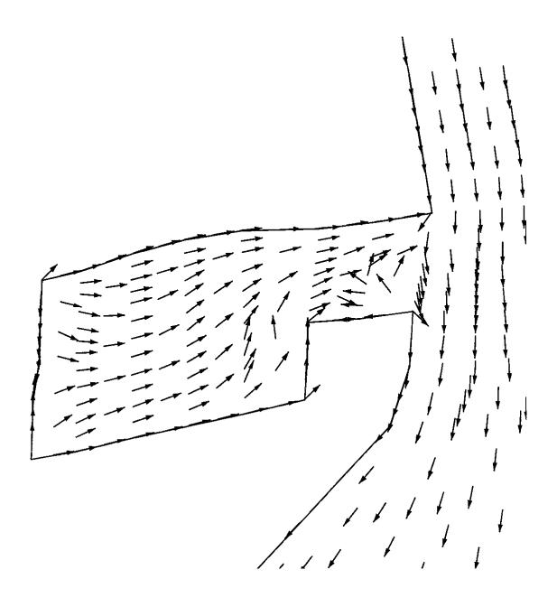
Figure 9.4 Constant Length (indicate flow direction only) Velocity Vectors in the Marina During Ebb Tide
