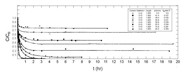
**Figure 3.11** Ratio C/C<sub>o</sub> versus Time for Kaolinite in Distilled Water (after Mehta and Partheniades 1975).
