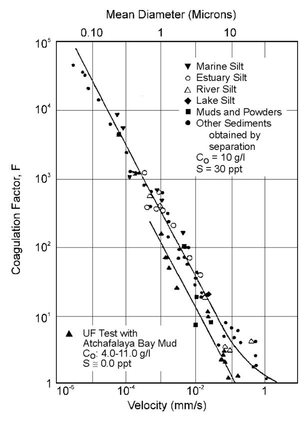
**Figure 3.18** Effect of Size and Settling Velocity of Elementary Particles on the Coagulation Factor of Natural Muds (after Bellessort 1973).
