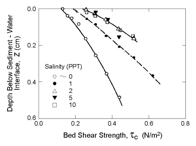
Figure 3.5 Bed Shear Strength Profiles as Functions of Salinity.
