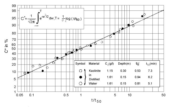
**Figure 3.14** C\* in Percent versus  $t/t_{50}$  for Kaolinite in Distilled Water (after Mehta and Partheniades 1975).
