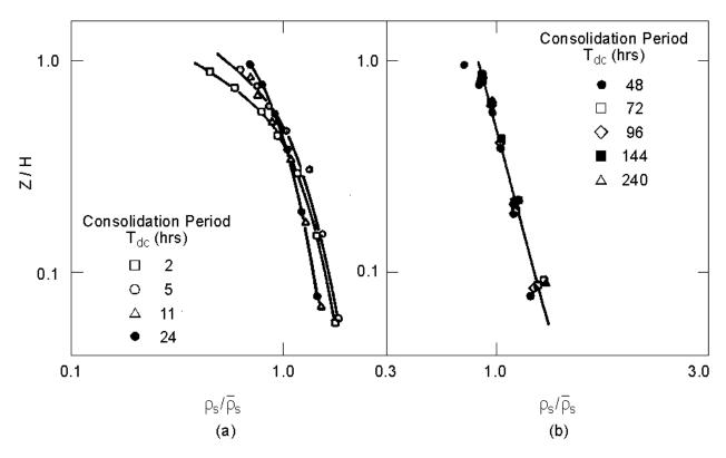
**Figure 3.24** Normalized Depth Below the Bed Surface versus Normalized Bed Bulk Density for Consolidation Times (a) Less than 48 Hours and (b) Greater than 48 Hours (after Dixit 1982).
