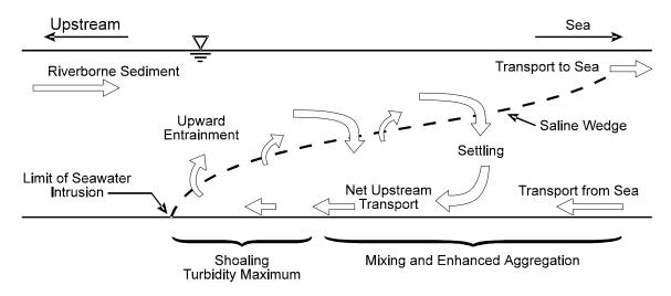
**Figure 3.2** Schematic Representation of Transport and Shoaling Processes in the Mixing Zone of a Stratified Estuary (after Mehta and Hayter 1981).
