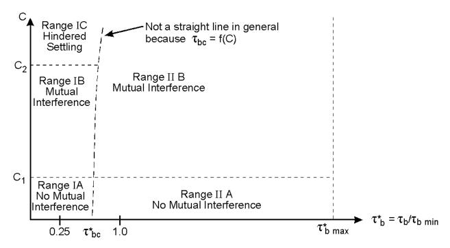
**Figure 5.3** Apparent Settling Velocity Description in Domains Defined by Suspended Sediment Concentration and Bed Shear Stress
