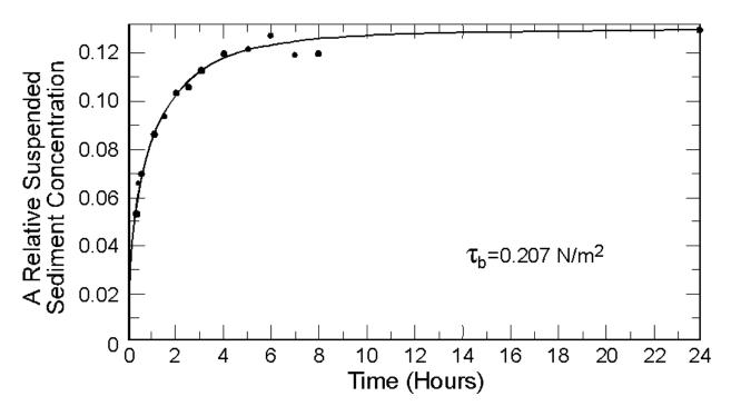
**Figure 3.6** Relative Suspended Sediment Concentration versus Time for a Stratified Bed (after Mehta and Partheniades 1979)
