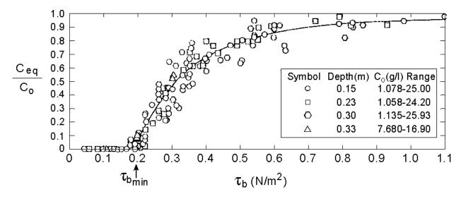
**Figure 3.12** Ratio  $C_{eq}/C_o$  versus Bed Shear Stress  $\tau_b$  (after Mehta and Partheniades 1975).
