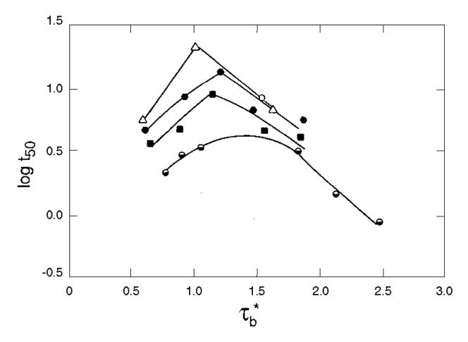
**Figure 3.15** Log  $t_{50}$  versus  $\tau_b^*$  for Kaolinite in Distilled Water (after Mehta and Partheniades 1975). 1973), hinders the upward flux of water expelled by consolidation of the lower suspension (Krone 1962).
