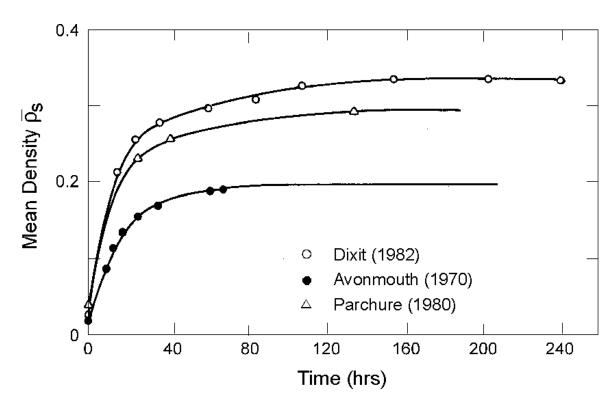
Figure 3.21 Variation of Mean Bed Density with Consolidation Time (after Dixit 1982).
