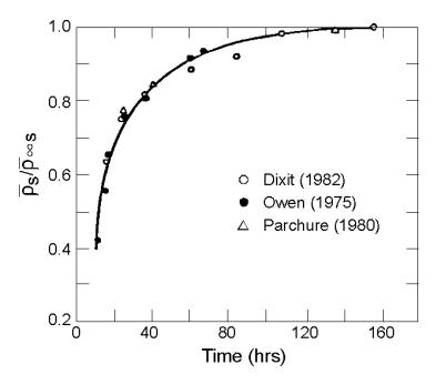
**Figure 3.22** Variation of the Normalized Mean Bed Density versus Consolidation Time (after Dixit 1982).
