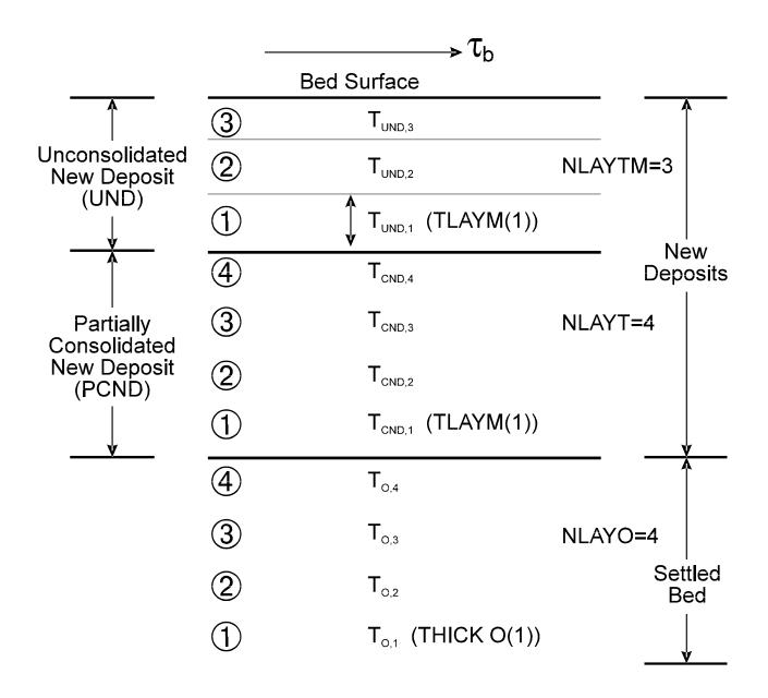
Figure 5.1 Bed Schematization Used in Bed Formation Algorithm
