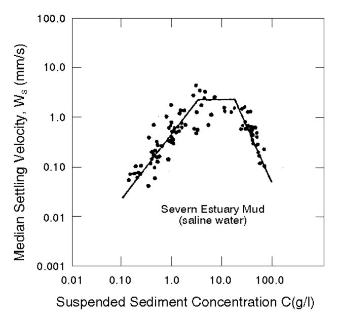
**Figure 3.17** Settling Velocity versus Concentration (after Thorn 1981). experiments (see Figure 3.16). Teeter (1983) found m to be less than 1.0 for sediment from Atchafalaya Bay, Louisiana.
