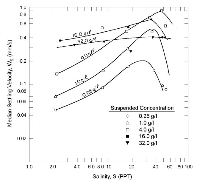
Figure 3.20 Effect of Salinity on Settling Velocity of Avonmouth Mud (after Owen 1970a).
