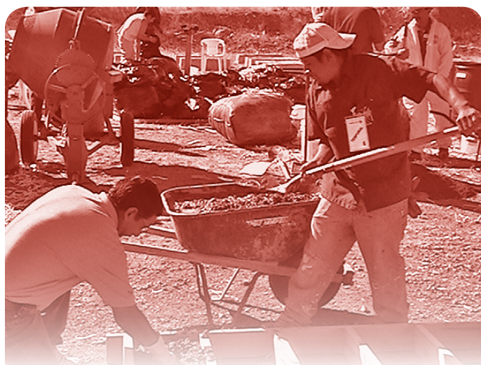
Teamwork by Nogales, Sonora, maquiladora workers produces hundreds of fibrous concrete blocks in a day.
