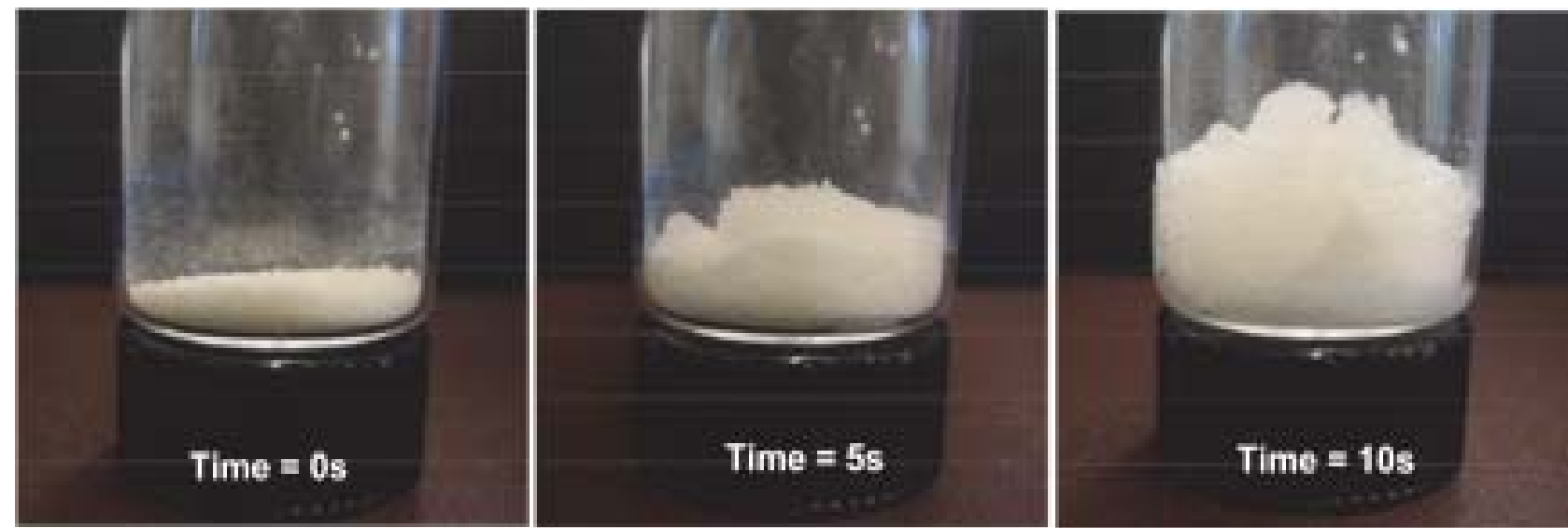
Above: Snapshot series of Osorb swelling when acetone is added drop-wise.
