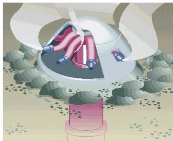
Figure 10c. The diffuser heads each disperse the effluent through eight ports.
