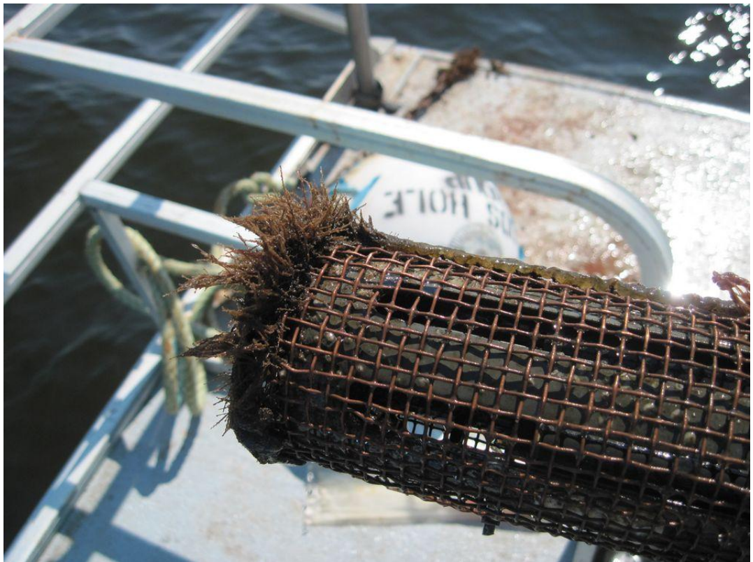
Figure 2. Biofouling (hydroids) on instrument 1000S in September 2012.
