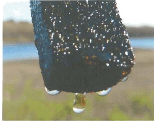
(b) water dripping from EMA sample while retaining oil.
