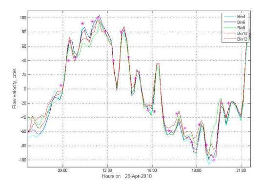
Figure 15. Long-channel flow velocity from selected HADCP bins for 28-Apr-10. Magenta stars (\*) show flow velocities (measured from the ADCP on the boat) used for estimation of sample volumes in the field during April 28th sampling.
