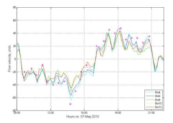
Figure 18. Long-channel flow velocity from selected HADCP bins for 07-May-10. Magenta stars show flow velocities (measured from the ADCP on the boat) used for estimation of sample volumes in the field May 7th sampling.
