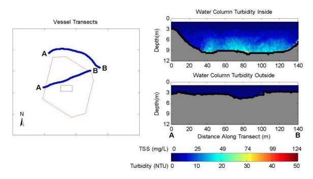
Figure 4-5. Observations from 50 to 53 Minutes after Release During May 27, 2009 Disposal into the New Bedford Harbor CAD Cell. The left panel shows concurrent inner and outer vessel transects. The right panel shows vertical slices of calibrated turbidity and TSS measured with ADCP along each vessel transect.
