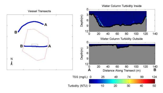
Figure 4-1. Observations Before Release During May 27, 2009 Disposal into the New Bedford Harbor CAD Cell. The left panel shows concurrent inner and outer vessel transects. The right panel shows vertical slices of calibrated turbidity and TSS measured with ADCP along each vessel transect.
