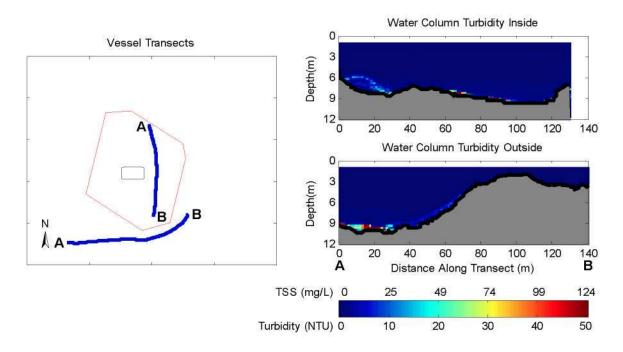
Figure 5-1. Observations Before Release During July 8, 2009 Disposal into the New Bedford Harbor CAD Cell. The left panel shows concurrent inner and outer vessel transects. The right panel shows vertical slices of calibrated turbidity and TSS measured with ADCP along each vessel transect.
