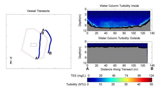
Figure 4-7. Observations from 63 to 67 Minutes after Release During May 27, 2009 Disposal into the New Bedford Harbor CAD Cell. The left panel shows concurrent inner and outer vessel transects. The right panel shows vertical slices of calibrated turbidity and TSS measured with ADCP along each vessel transect.
