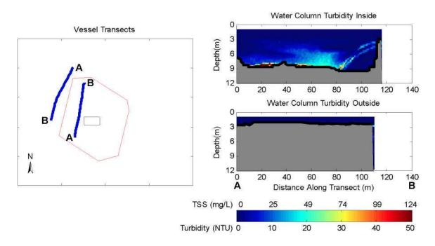
Figure 5-5. Observations from 26 to 29 Minutes after Release During July 8, 2009 Disposal into the New Bedford Harbor CAD Cell. The left panel shows concurrent inner and outer vessel transects. The right panel shows vertical slices of calibrated turbidity and TSS measured with ADCP along each vessel transect.
