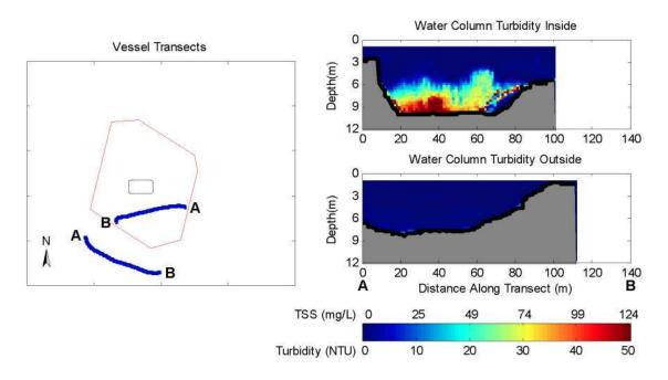
Figure 2-3. Observations from 10 to 12 Minutes after Release During May 20, 2009 Disposal into the New Bedford Harbor CAD Cell. The left panel shows concurrent inner and outer vessel transects. The right panel shows vertical slices of calibrated turbidity and TSS measured with ADCP along each vessel transect.
