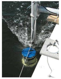
Figure 2. ADCP Mounted in Operational Position Over the Side of the Sea Quest with the Acoustic Transducers Just Below the Water Surface.
