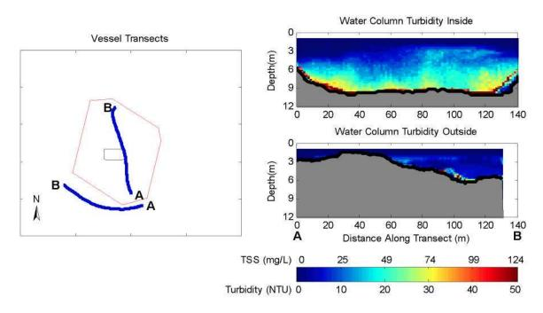
Figure 2-5. Observations from 39 to 43 Minutes after Release During May 20, 2009 Disposal into the New Bedford Harbor CAD Cell. The left panel shows concurrent inner and outer vessel transects. The right panel shows vertical slices of calibrated turbidity and TSS measured with ADCP along each vessel transect.
