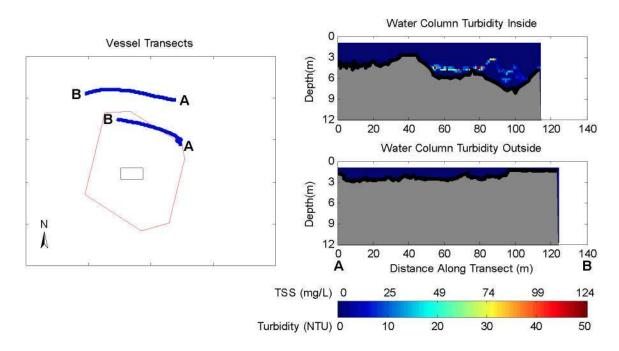
Figure 1-1. Observations Before Release During April 14, 2009 Disposal into the New Bedford Harbor CAD Cell. The left panel shows concurrent inner and outer vessel transects. The right panel shows vertical slices of calibrated turbidity and TSS measured with ADCP along each vessel transect.
