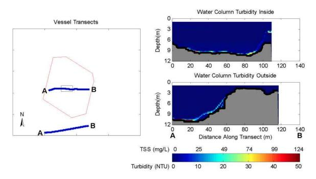
Figure 3-1. Observations Before Release During May 21, 2009 Disposal into the New Bedford Harbor CAD Cell. The left panel shows concurrent inner and outer vessel transects. The right panel shows vertical slices of calibrated turbidity and TSS measured with ADCP along each vessel transect.
