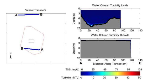
Figure 1-5. Observations from 40 to 44 Minutes after Release During April 14, 2009 Disposal into the New Bedford Harbor CAD Cell. The left panel shows concurrent inner and outer vessel transects. The right panel shows vertical slices of calibrated turbidity and TSS measured with ADCP along each vessel transect.
