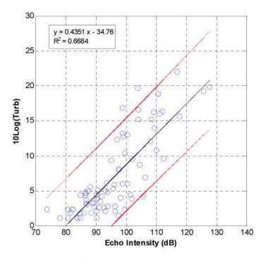
Figure 7. Least Squares Regression Analysis of Turbidity from Whole Water Samples Analyzed in the Laboratory versus ADCP Echo Intensity in Decibels (dB). Red Lines Indicate the Regression 95% Confidence Interval.
