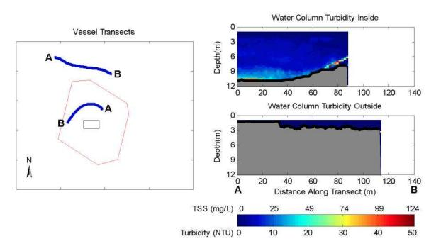
Figure 1-3. Observations from 19 to 22 Minutes after Release During April 14, 2009 Disposal into the New Bedford Harbor CAD Cell. The left panel shows concurrent inner and outer vessel transects. The right panel shows vertical slices of calibrated turbidity and TSS measured with ADCP along each vessel transect.
