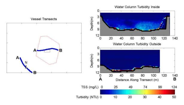
Figure 3-5. Observations from 39 to 42 Minutes after Release During May 21, 2009 Disposal into the New Bedford Harbor CAD Cell. The left panel shows concurrent inner and outer vessel transects. The right panel shows vertical slices of calibrated turbidity and TSS measured with ADCP along each vessel transect.
