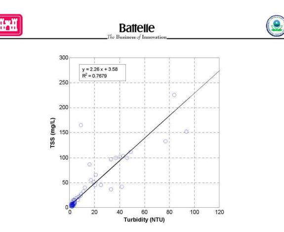
Figure 6. Least Squares Regression Analysis of TSS versus Turbidity from Whole Water Samples Analyzed in the Laboratory.
