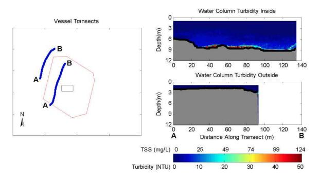
Figure 5-7. Observations from 58 to 61 Minutes after Release During July 8, 2009 Disposal into the New Bedford Harbor CAD Cell. The left panel shows concurrent inner and outer vessel transects. The right panel shows vertical slices of calibrated turbidity and TSS measured with ADCP along each vessel transect.
