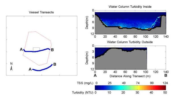
Figure 2-7. Observations from 84 to 87 Minutes after Release During May 20, 2009 Disposal into the New Bedford Harbor CAD Cell. The left panel shows concurrent inner and outer vessel transects. The right panel shows vertical slices of calibrated turbidity and TSS measured with ADCP along each vessel transect.
