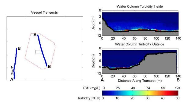
Figure 3-7. Observations from 57 to 59 Minutes after Release During May 21, 2009 Disposal into the New Bedford Harbor CAD Cell. The left panel shows concurrent inner and outer vessel transects. The right panel shows vertical slices of calibrated turbidity and TSS measured with ADCP along each vessel transect.
