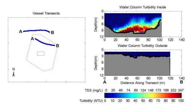
Figure 4-3. Observations from 5 to 9 Minutes after Release During May 27, 2009 Disposal into the New Bedford Harbor CAD Cell. The left panel shows concurrent inner and outer vessel transects. The right panel shows vertical slices of calibrated turbidity and TSS measured with ADCP along each vessel transect. Note change in turbidity scale.
