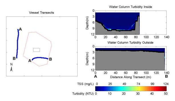
Figure 2-1. Observations Before Release During May 20, 2009 Disposal into the New Bedford Harbor CAD Cell. The left panel shows concurrent inner and outer vessel transects. The right panel shows vertical slices of calibrated turbidity and TSS measured with ADCP along each vessel transect.
