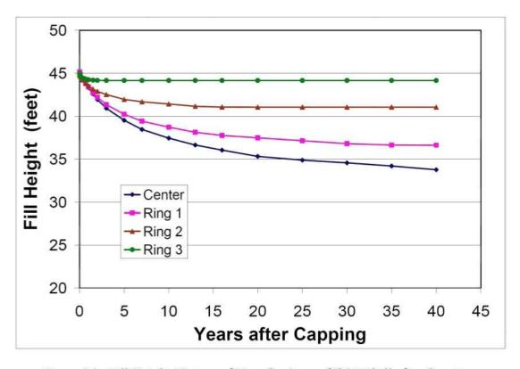
Figure 14. Fill Height History of Four Sections of CAD Cell after Capping.
