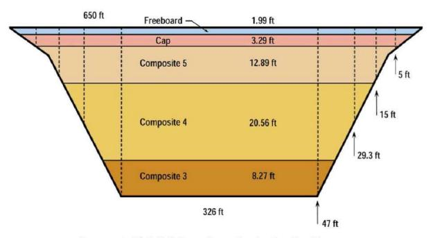
Figure 15. CAD Cell Status Immediately after Cap Placement.
