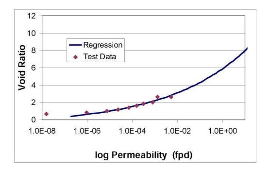
Figure 9. Void Ratio vs. Effective Stress and Void Ratio vs. Permeability Relationships for New Bedford Harbor Sediment Composite 3.
