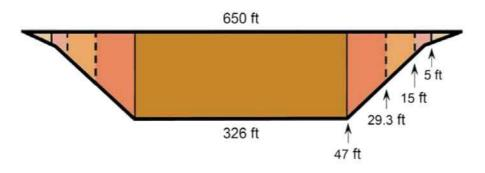
Figure 12. Schematic of CAD Cell Sections for PSDDF and CAP Modeling.
