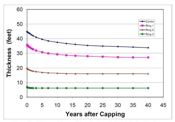
Figure 22. Thickness History of Four Sections of CAD Cell after Capping.
