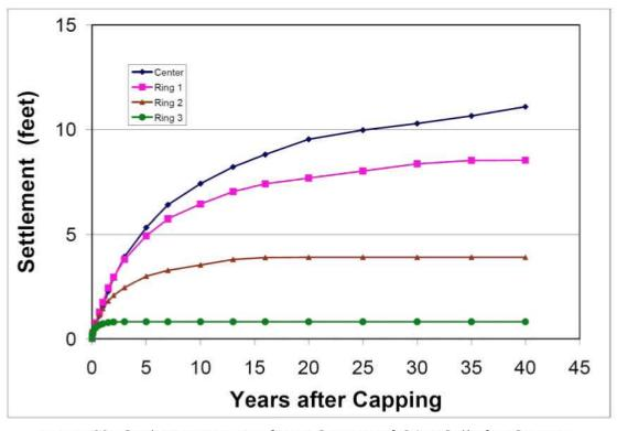
Figure 23. Settlement History of Four Sections of CAD Cell after Capping.
