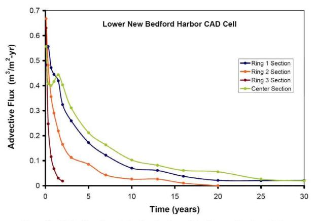
Figure 21. Water Flux through the Four Sections of the Cap as a Function of Time.
