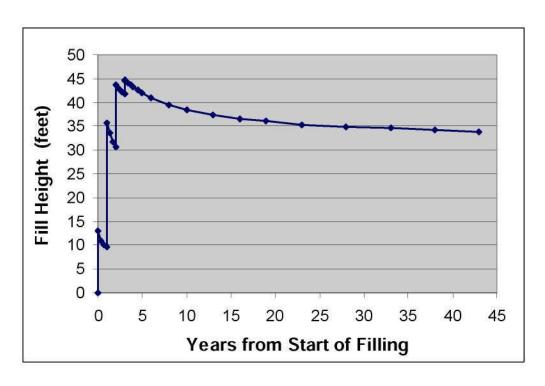
Figure 13. Fill Height History of Center Section of Lower New Bedford Harbor CAD Cell.
