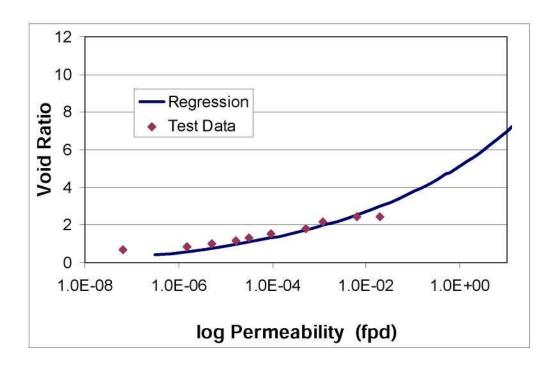
Figure 10. Void Ratio vs. Effective Stress and Void Ratio vs. Permeability Relationships for New Bedford Harbor Sediment Composite 4.
