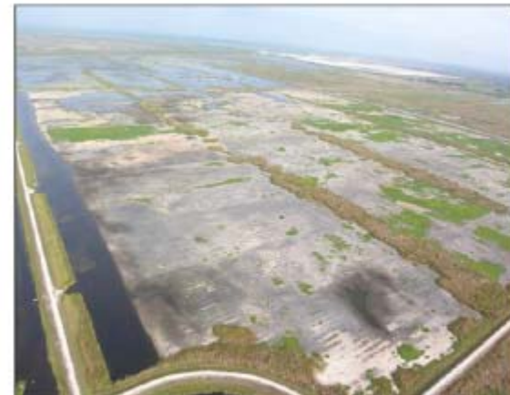
Figure 5-20. An aerial photo of STA-1E, Cell 4N, in May 2009, showing cell dryout, resulting in loss of submerged aquatic vegetation (SAV) (photo by the SFWMD).
